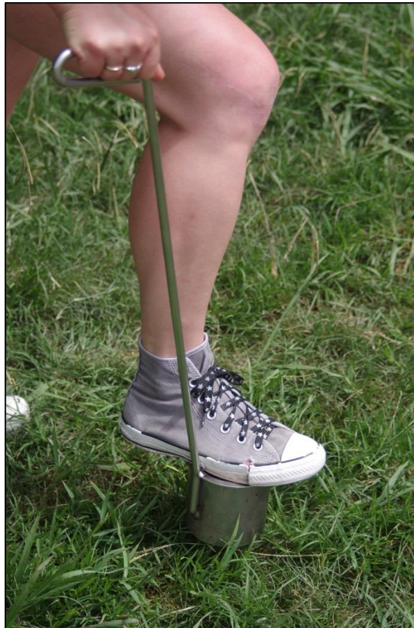
Figure 3.1: Soil samples were collected by using a bucket core sampler (February, 2016).
