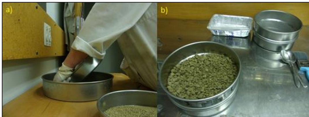
Figure 3.3: a) Crushing soil aggregates in metal tins. b) Sieving soil aggregates to <2 mm size for analysis (June 2015).
