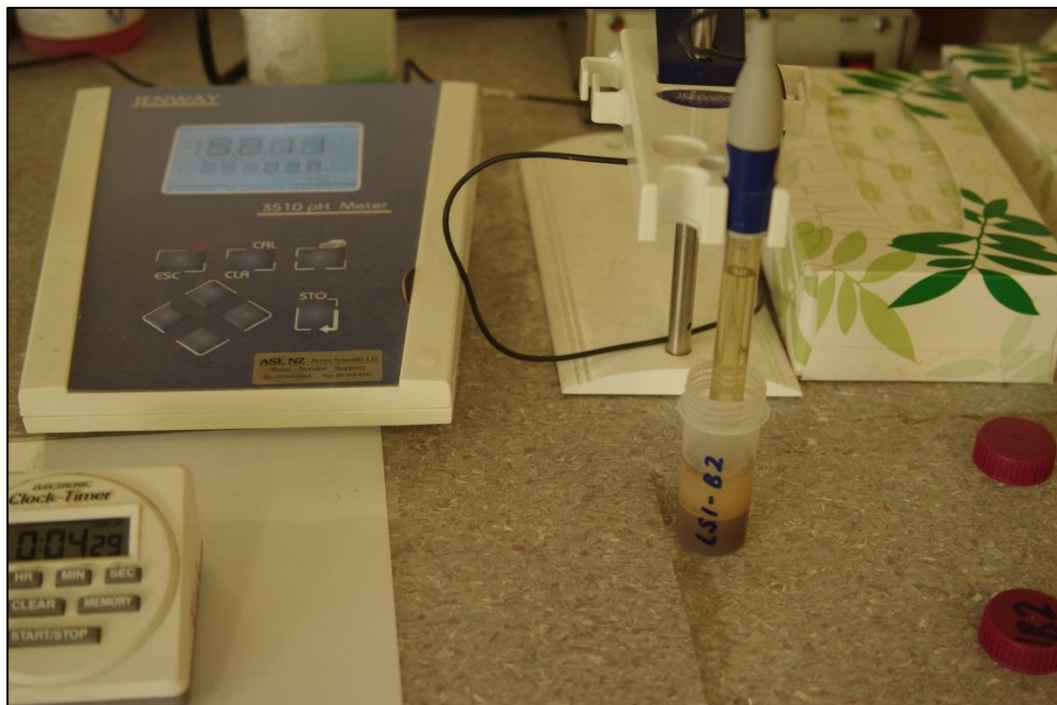
Figure 3.7: Measuring soil pH following the settling period of 24 hours using the Jenway (3510) pH electrode probe.
