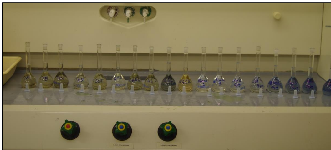
Figure 3.5: Samples and standards in the fumehood, as colour development was occurring during a trial run of Olsen P testing (August 2015).
