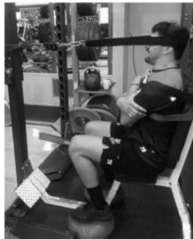
Figure 1. Illustration of the isometric neck strength test experimental setup for extension.
