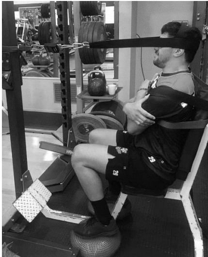
Figure 5. Illustration of the isometric neck strength test experimental setup for extension.
