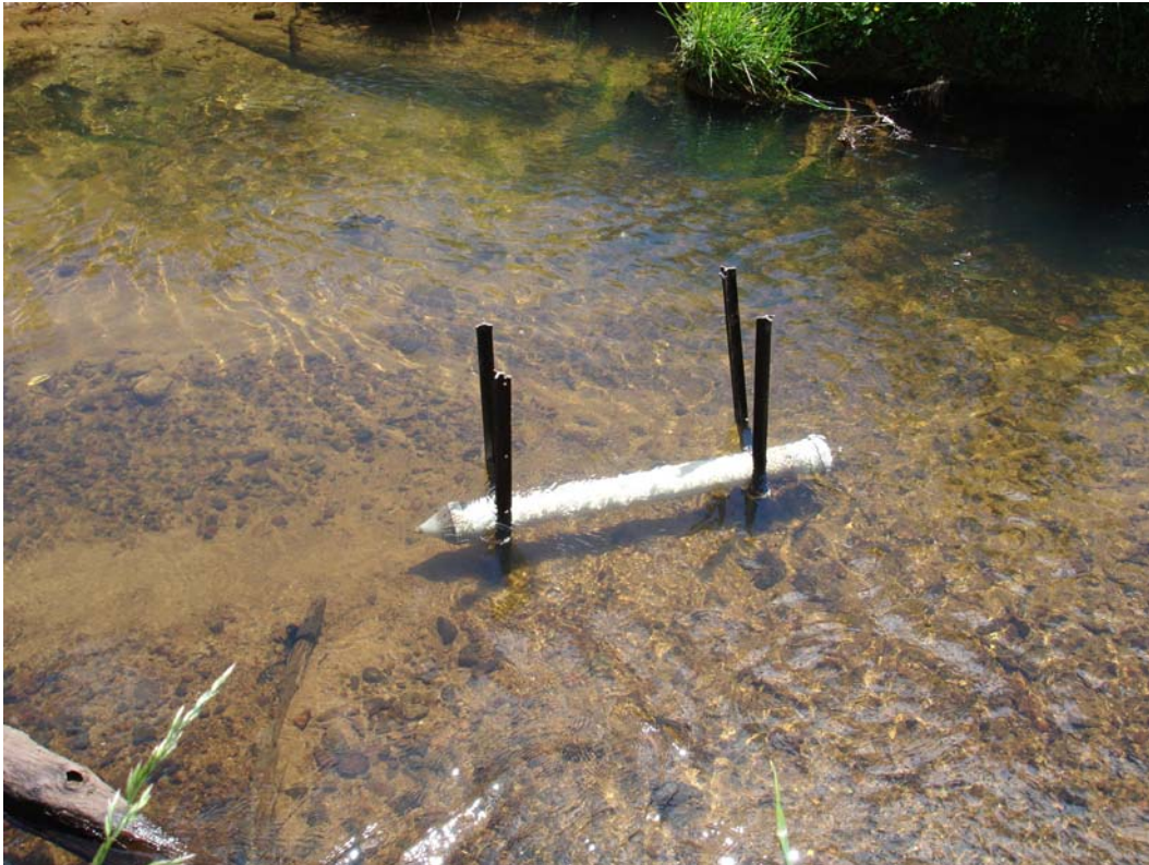
Figure 5.4. A) Schematic drawing of the time integrated sediment sampler; B) field deployment of the time integrated sediment sampler in the Waitekuri River.
