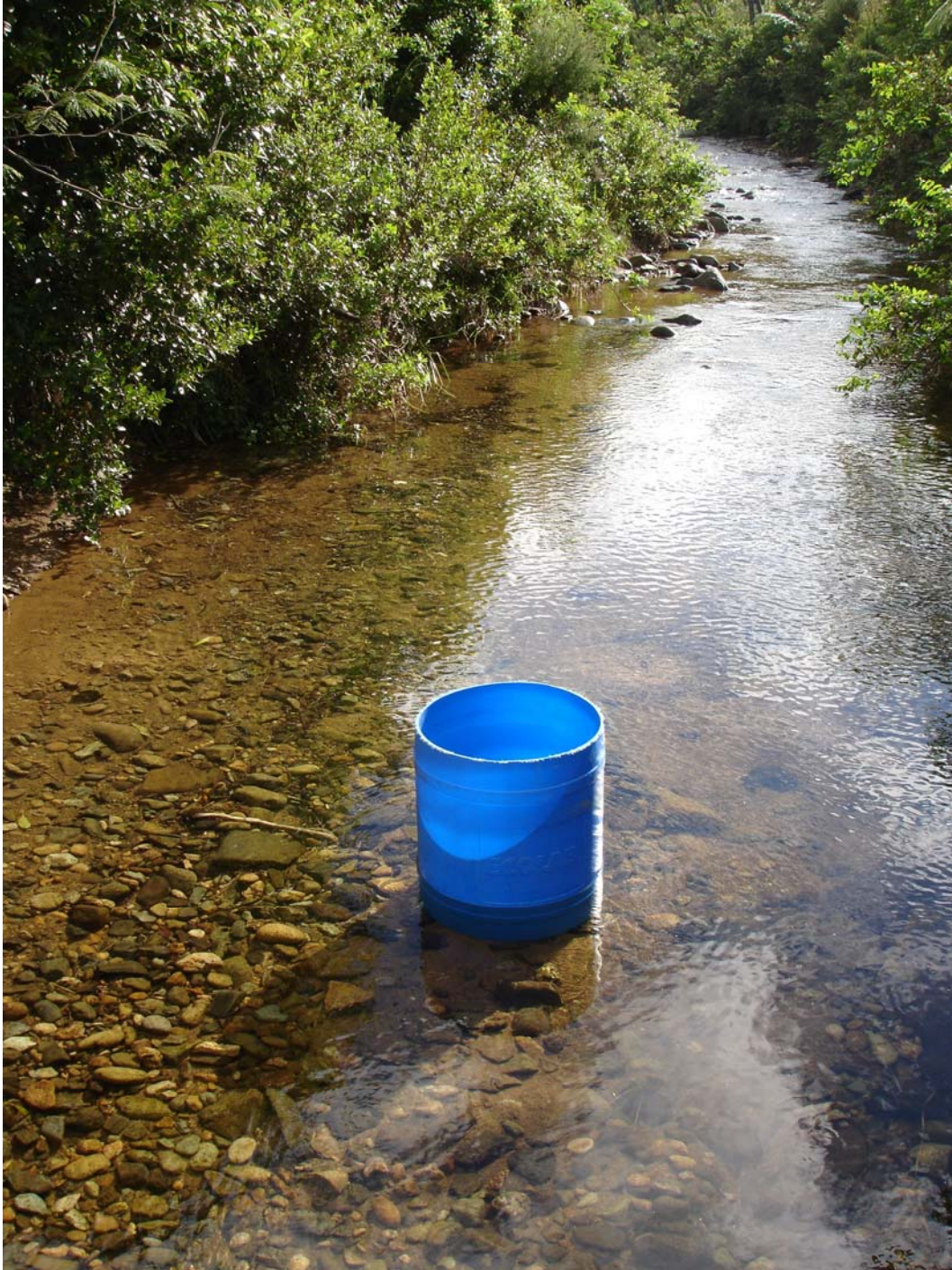
Figure 10.1. Sampling drum used for stream sediment storage estimation.
