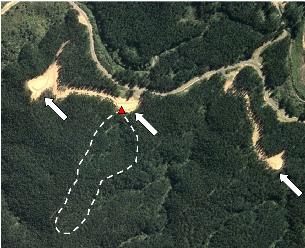
Figure 8.4. Location of the EX-H6 subcatchment off State Highway 26. The approximate catchment area is marked and the monitoring site is indicated by a red triangle. The image is taken before harvesting. Log landings constructed in preparation for logging operations can be seen (arrows).
