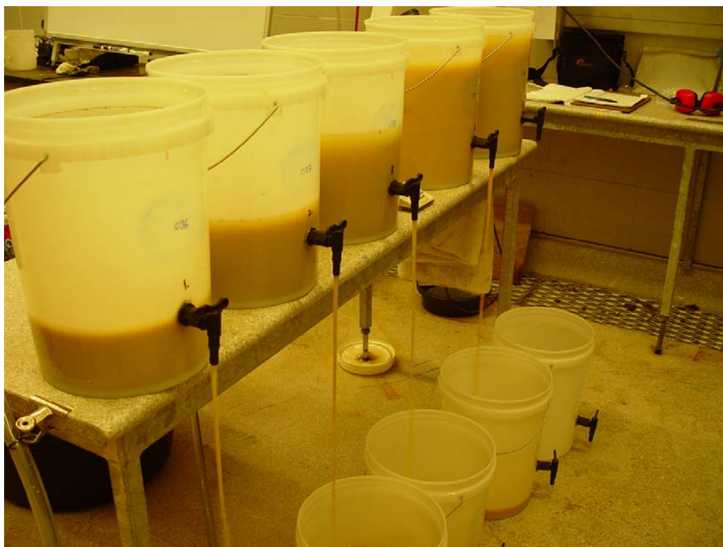
Figure 4.2. Picture of the settling method where the sediment is stirred in 20 L buckets and the desired fraction is recovered by drawing off the fraction still in suspension in the 25 cm fall zone.
