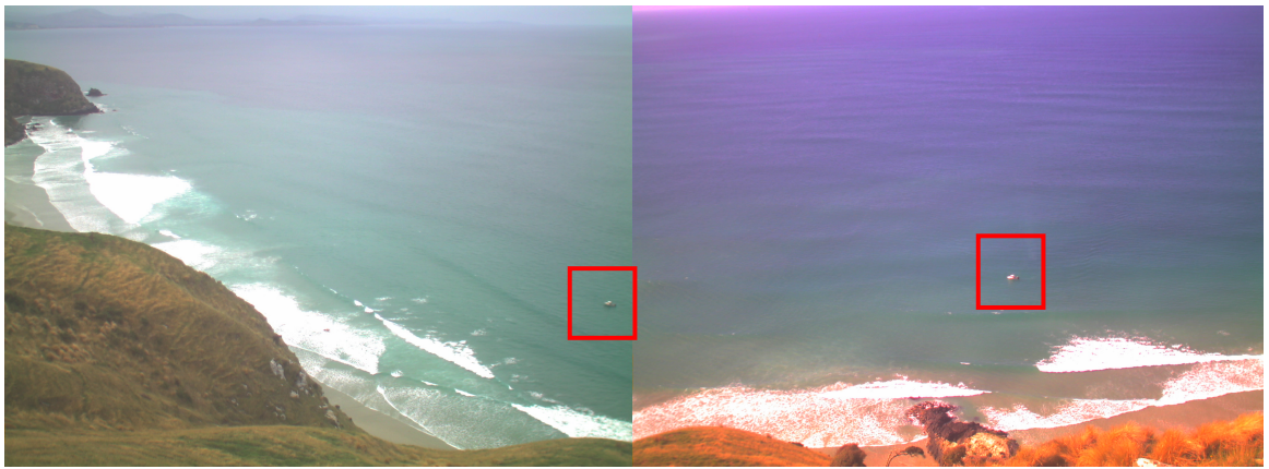
Figure 3-2 Image depicts GCPs being collected along Aramoana Beach on the 11 th March 2015 by a POL boat. The left panel is an image snapped by Camera 1 at Aramoana and the right panel is an image snapped by Camera 2 at Aramoana. Note: the red boxes indicate the position of the survey boat.
