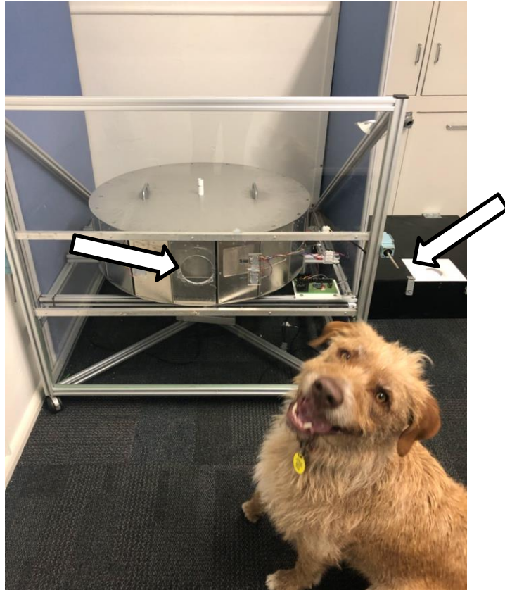
Figure 4. Rusty sitting in front of the port of the apparatus (lined with grey tape). The lever is attached to the frame of the apparatus (right).
