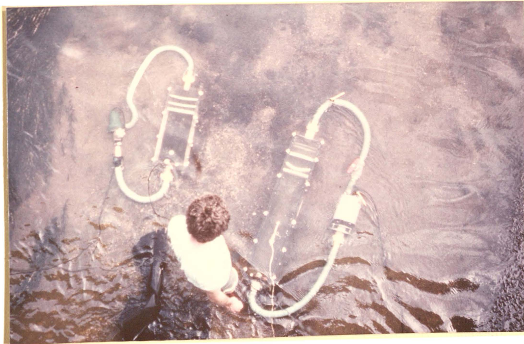
Plate 4.2 Large and small benthic chamber systems installed on the Waitoa River at Walton Bridge, February 1983
