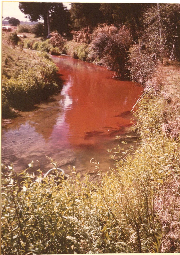
Plate 3.5 Dye study in the Waitoa River 50 m below Waharoa discharge showing 'sewage fungus' proliferation, 16 February 1982.
