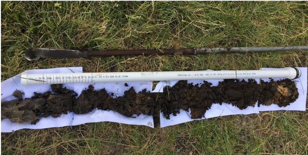
**Figure 8: Equipment used for piezometer installation. Metal hand auger (top), plastic tubing (middle), and screen and soil log taken from drilling (bottom).**
