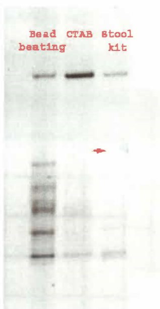
Figure 3.1 DGGE gel of MVS4 transect environmental sample 4.1. Bacterial 16S rDNA extracted using bead-beating, CTAB and QIAmp DNA Stool Mini Kit methods of DNA extraction.
