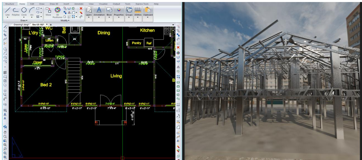
Figure B.1: FrameCAD Structural Plan and Blender 3D Model Render.
