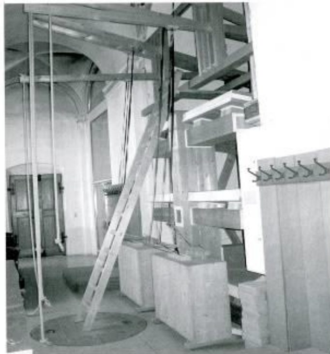
Plate 3.9: Katholischen-Stadtkirche-St. Alexander, Rastatt. Reconstruction of the wind system of the Stieffell-Orgel, Photographic image, 2007. 49
