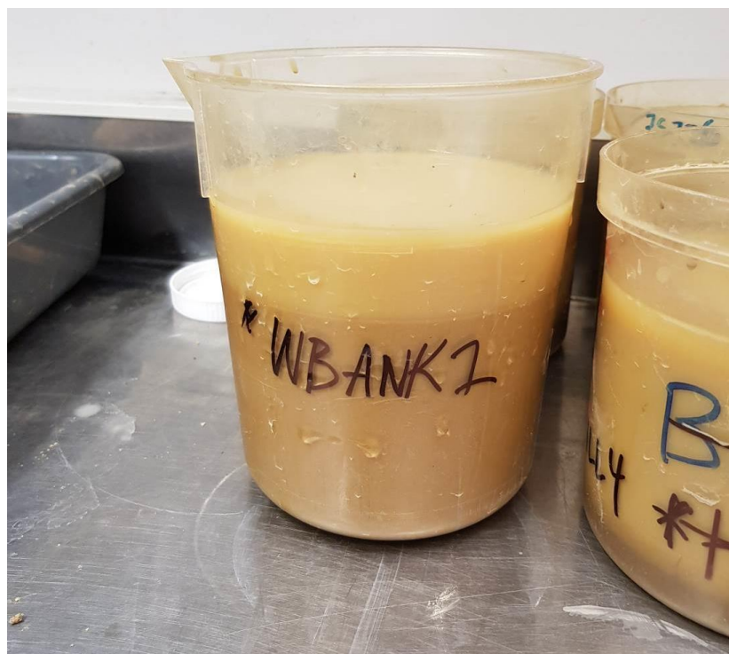
Figure 4.11. Example of a wet sieved stream bank soil sample ( <63\mu\text{m} ), 20 minutes after sieving and shows the sediment beginning to settle in the bottom of the beaker.
