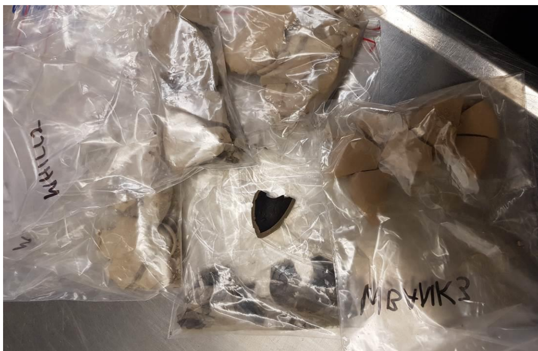
Figure 4.13. A hillslope soil sample from the Whakakai catchment (WHILL1 Appendices Table A.1) that developed a dark black colour post drying in the 60°C oven, compared to other stream bank and hillslope samples from the Whakakai catchment, which had a light brown colour post drying.
