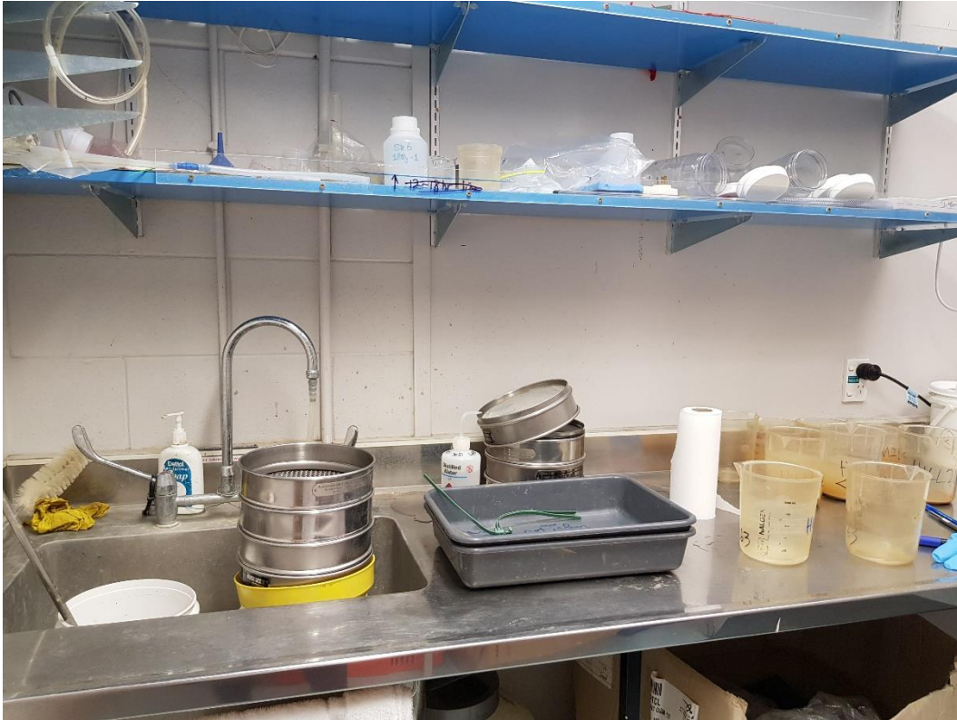
Figure 4.9. Wet sieving area in the laboratory, showing sieves ranging from 4mm to <63 \mu\text{m} .
