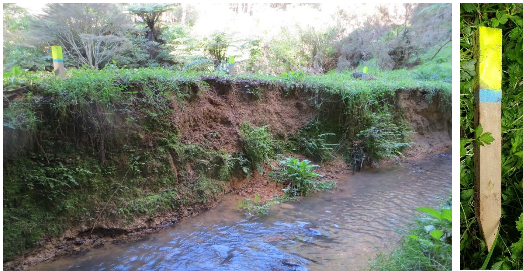
Figure 3.4. Example of on 3D modelling bank sites (left). Close up of marked garden stakes used for scale during the creation of the 3D models (right).
