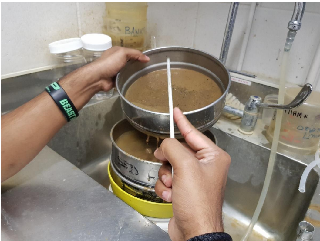
Figure 4.10. Wet sieving a suspended sediment sample (sampler near the left bank) in the Mangaotama catchment.
