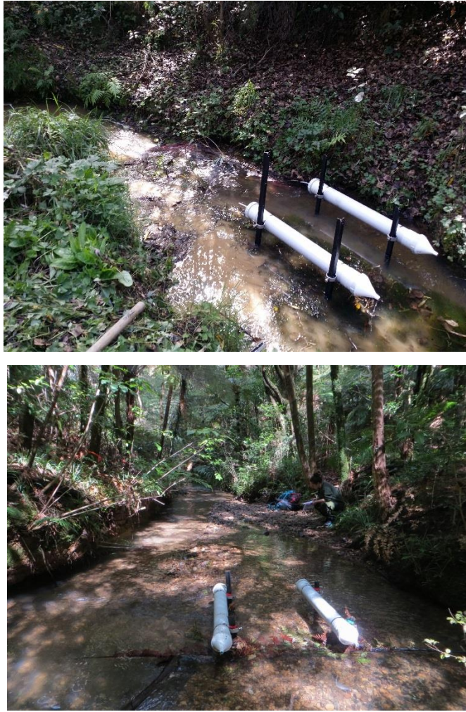
Figure 4.6. Phillips samples in the Mangaotama (top) and Whakakai catchment (Photo: M. Balks, 2018) (bottom) installed 15cm above base flow. N.B. The photograph was taken after the samplers were re-installed ~40m from the NIWA monitoring station on July 13.
