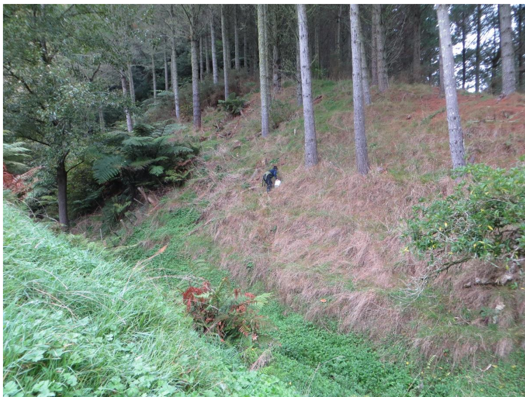
Figure 4.3. Soil sample collection from a hillslope site under pine plantation in the Mangaotama catchment. Soil samples were collected in a semi-straight transect from the bottom of the hill to the top of the hill, and more samples were taken at the apex of the hill (Photo: K. Huirama, 2018).
