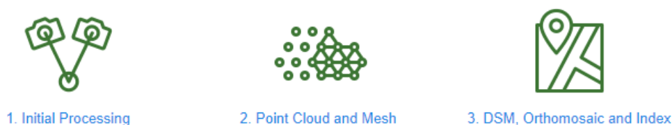
Figure 3.6. Chart showing the processing steps used by the Pix4D software to create 3D models from terrestrial based imagery (Pix4D, 2017).
