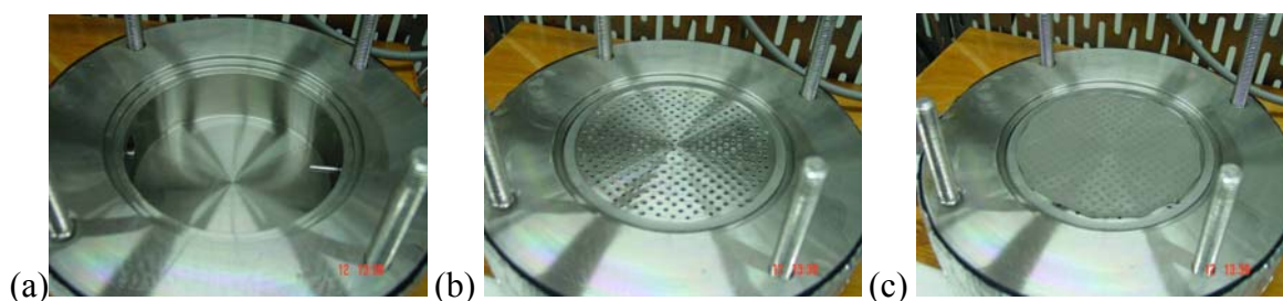
Figure 4:07 Membrane unit (a) permeate chamber, (b) perforated plate, (c) wire gauze.
