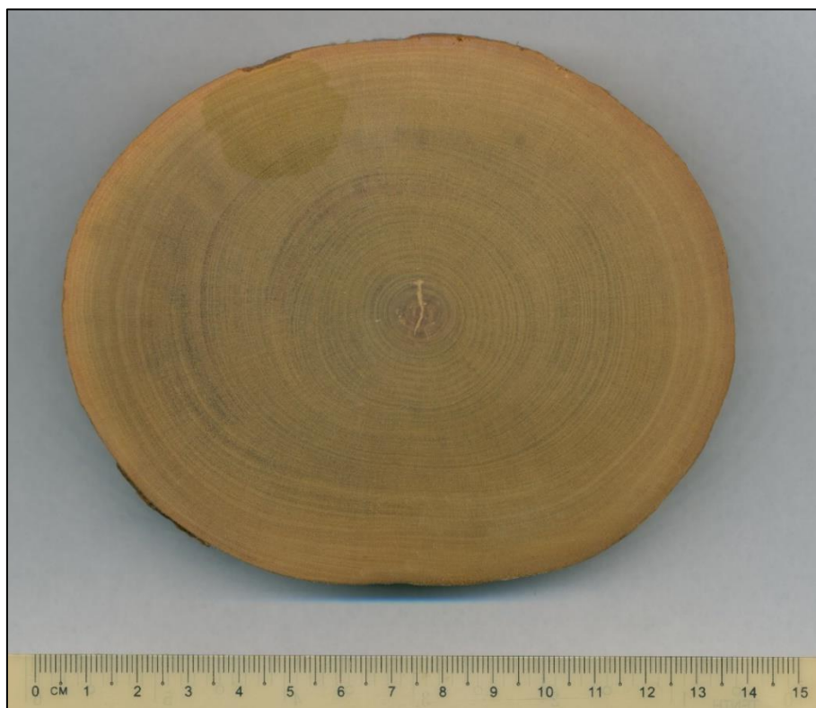
Figure 5.2.1. Example of a post sample cut, sanded and bleached for tree-ring analysis.
