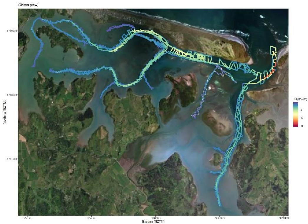
Figure 9: Extent of bathymetric survey undertaken by Dean Sandwell and Megan Raiapa at the University of Waikato in 2019.
