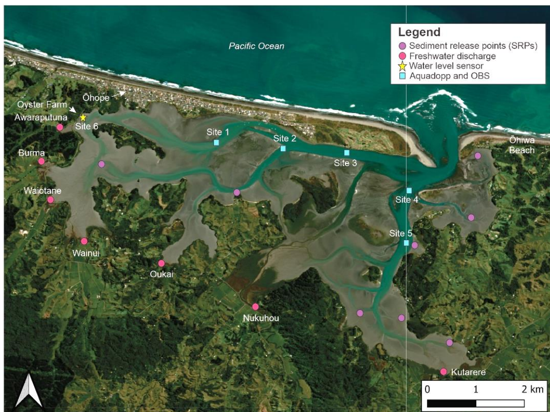
Figure 1: Field site including deployment locations and the location of stream inflows (background image is from Sentinel-2 satellite data).
