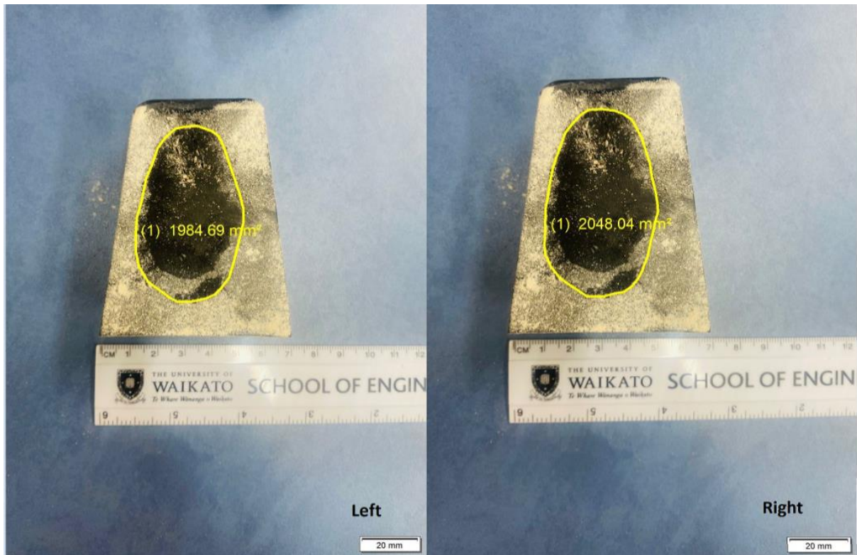
Figure 4-16: Shows the obtained surface area by the 1 mm infill gyroid infilled fingers
