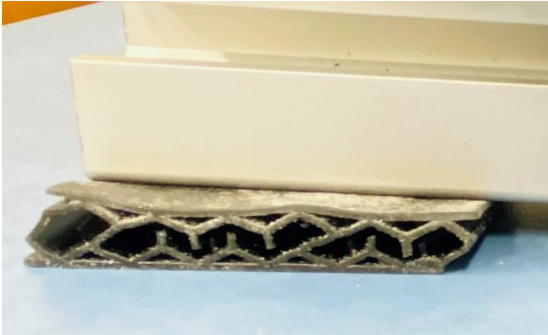
Figure 4-7: Shows buckling of honeycomb under load
