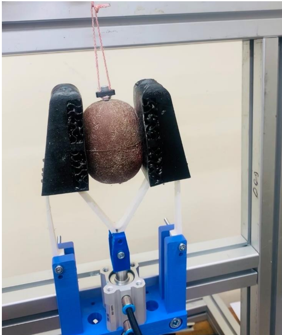
Figure 4-15: Shows the grasping fake kiwifruit with a rubber gripper
