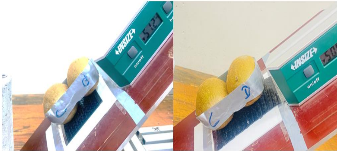
Figure 3-9 Shows the coefficient of friction using textured surfaces and real kiwifruits
