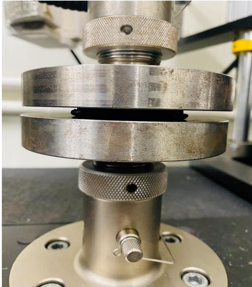
Figure 4-5: Shows the compression testing of lattice structures in an Instron machine
