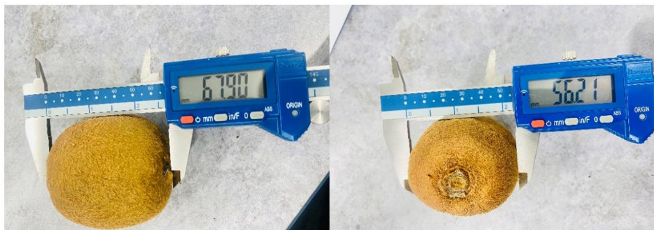
Figure 3-1: Measuring length and diameter of kiwifruit using digital vernier calliper
