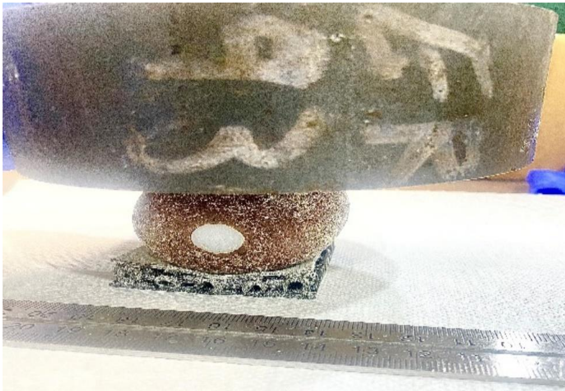
Figure 4-9: Applying a 60 N load to the kiwifruit to compress the 3D printed sample.
