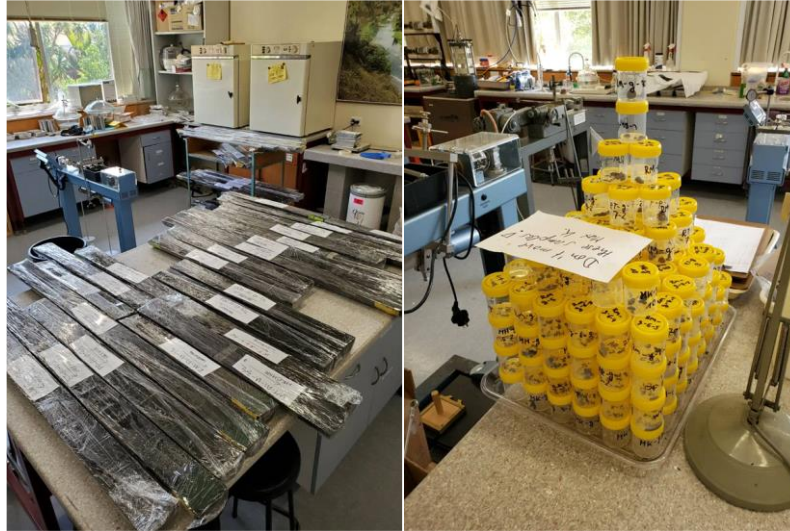
Fig. 2.5. Left: 19 sediment cores cut and logged. Right: Samples taken from the cores, awaiting physical and geotechnical properties analyses
