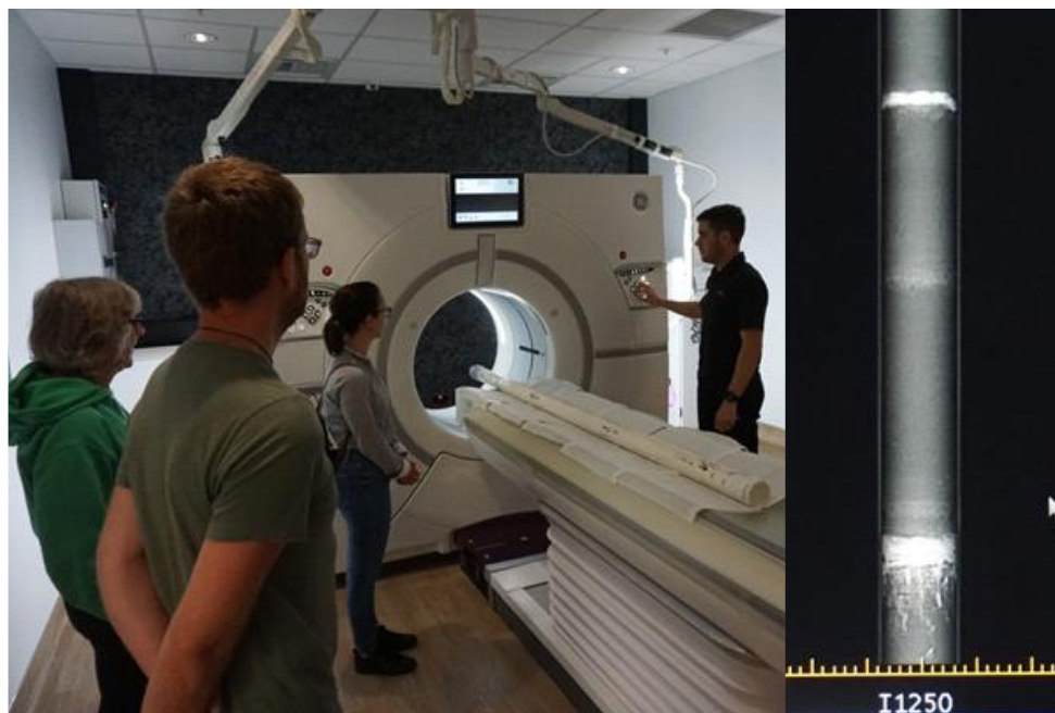
Fig. 2.4. Left: Sediment cores being scanned using a new medical CT scanner at Hamilton Radiology. Right: X-ray image of a sediment core, live in Hamilton radiology, showing SSDS in a tephra layer
