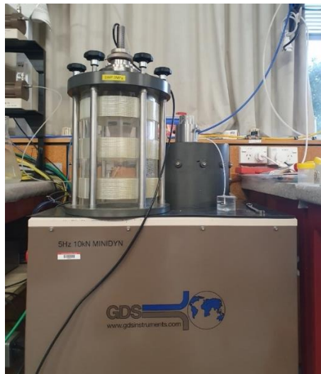
Fig. 2.5. GDS Advanced Dynamic Triaxial Equipment at the University of Waikato
