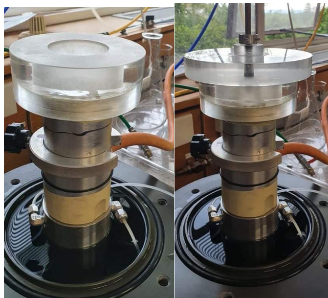
Fig. 2.6. Membrane protection collar (left) and full moist tamping guidance (membrane protection collar, guidance collar and tamper) assembled (right) as per Ladd (1978)
