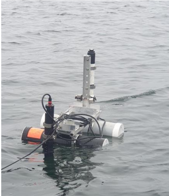
Figure 3.3. Satlantic HyperOCR with downwelling irradiance sensor (top right) and upwelling radiance sensor (bottom left) deployed in Lake Rotomā.
