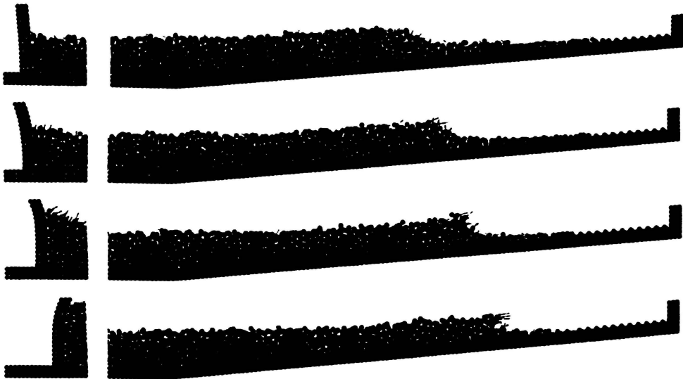
Figure 2.24: An example of a breaking wave generated by Koshizuka et al. (1998) using their MPS model. A large section of the domain has been removed for these images but the wave making section remains at the left. The arrows are velocity vectors.
