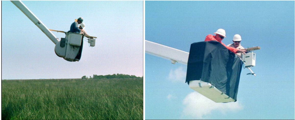
Figure 13: Collection of spectra above the canopy of salt marsh (left) and calibrating the spectrometer using a Spectralon reflectance standard for reference. A dark cloth is used on the bucket to suppress scattered light.
