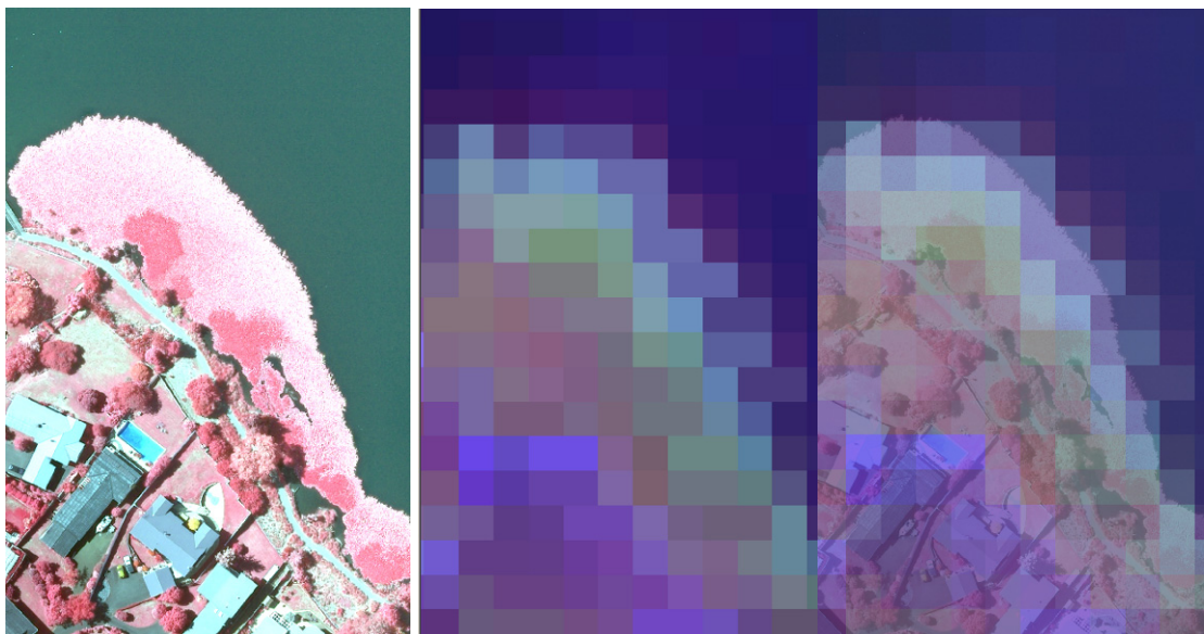
Figure 11: A close-up of VHSR image (left) showing water lily community on Hamilton lake, SPOT-5 XS data of the same site (middle), and display of SPOT XS data with QB (right) that determines sub-pixel proportion of the corresponding mixed features
