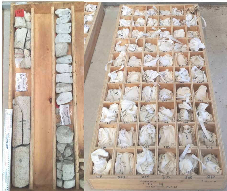
Fig. 4.1. Examples of cut core section where core samples were collected from and rock cuttings at 5 m intervals in cloth bags where samples were taken every 20 m.
