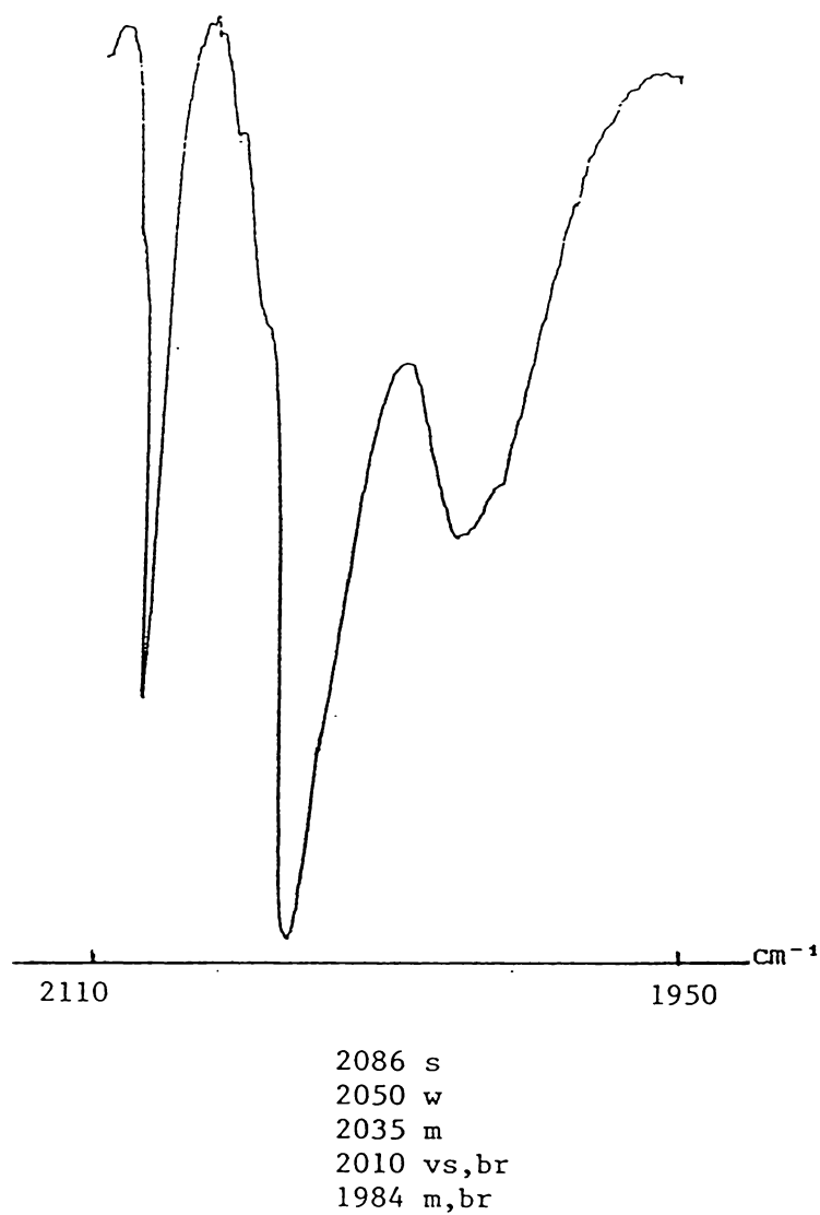
Figure 7.2. Infrared active carbonyl stretches of the product of reaction between \text{Et}_4\text{NSnCl}_3 and \text{Me}_3\text{SnCo(CO)}_4 . Recorded in \text{CH}_2\text{Cl}_2 .
