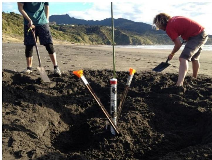
*Photo A-3. Upper photo: designed tubes for installing in Solinst piezometers locations (longer tube for high tide piezometers and shorter ones for low tide piezometers). Middle and lower photos: high tide tube deployment in the second and third transects respectively.*
