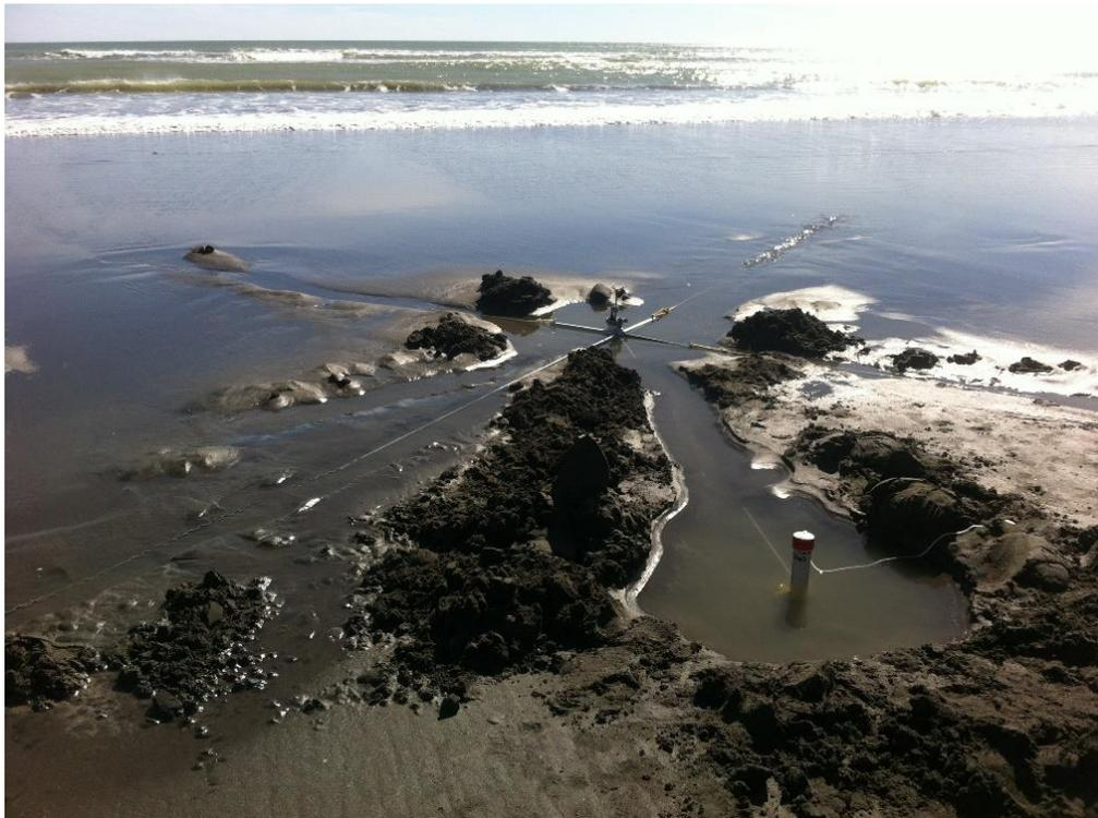
*Photo A-5. Location of the ADV, which was buried in the swash zone close to the low tide Solinst piezometer in the second and third transects.*
