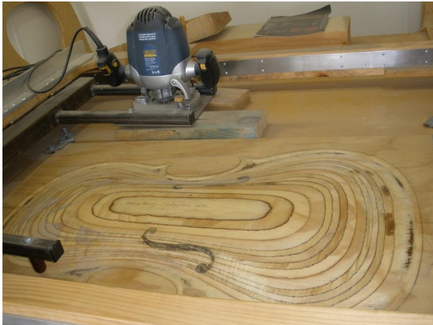
Plate 17: The router is used to automatically carve down the first stages of some of the instruments.
