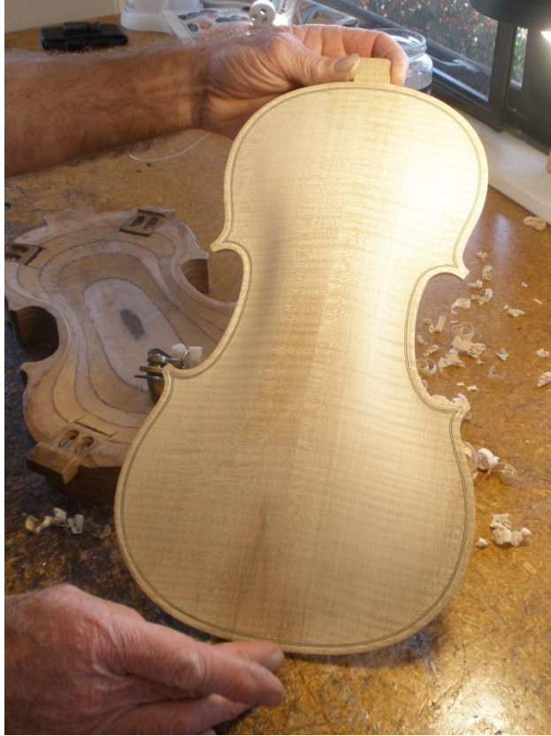
Plate 19: The outside. Also visible is the wooden mould within which the body of the instrument is secured during the carving down.
