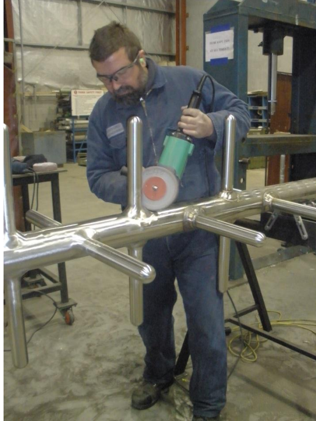
Plate 38: Jeff polishing the mixing mechanism for a pharmaceutical blending machine. In this instance, the part was being polished in the main workshop because of it was too large to fit in the polishing room.
