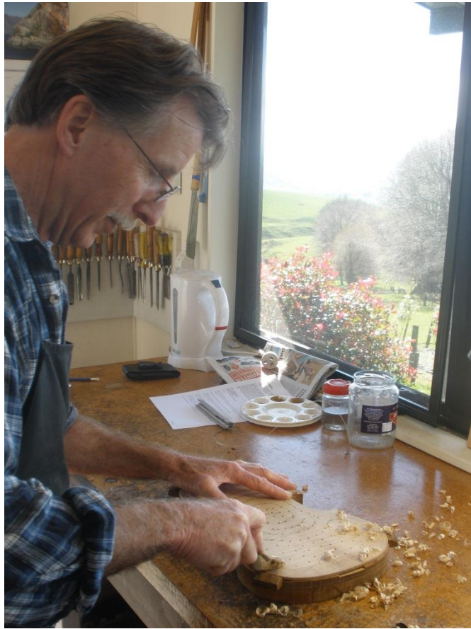
Plate 18: Using a small thumb plane for the early carving down stage (inside) for a replica Sanctus Seraphin violin (origin Venice 1746).
