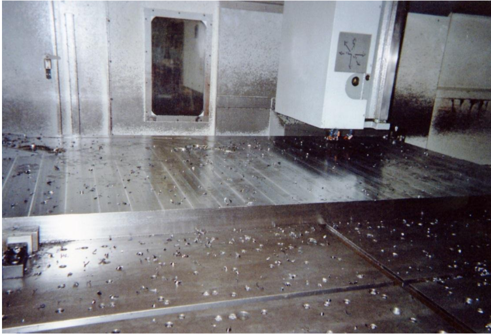
Plate 46: The slab is fixed in place. Milling has just begun on this half of the mould. The large white box-like structure holds the movable milling head.
