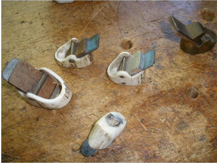
Plate 15: Handmade deer horn and metal file thumb planes. The bottom one is upside-down and shows the cutting edge while that on the right is manufactured from metal.
