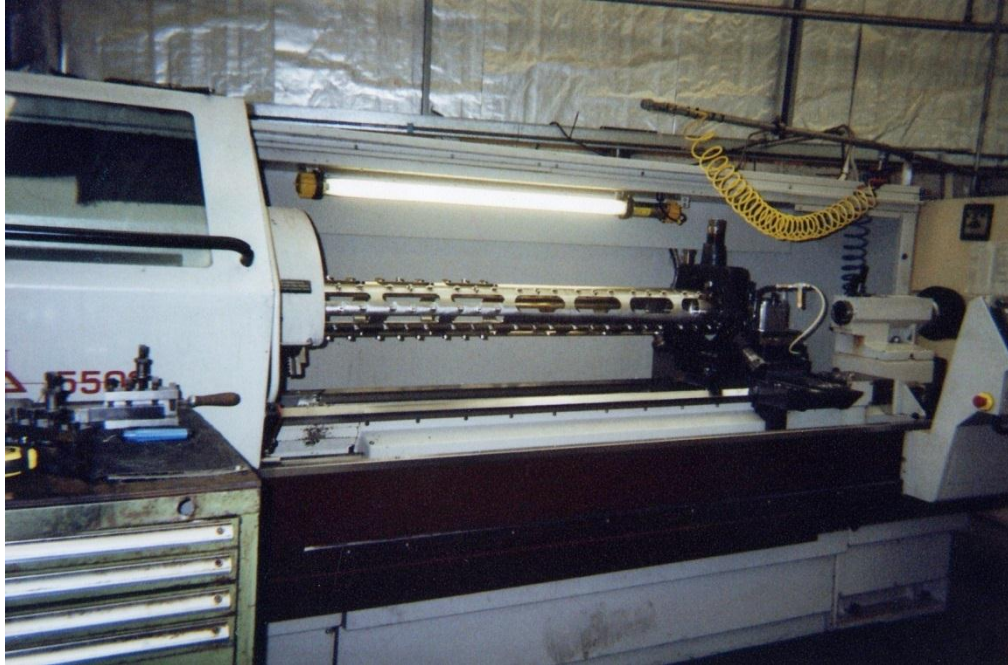
Plate 28: The Alpha lathe with a mixing dasher held between the chuck and the tailgate.
