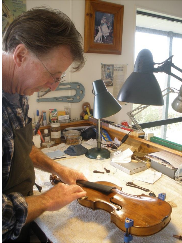
Plate 20: Noel restoring a Mougnot violin (origin Rouen 1789) – the polishing process.
