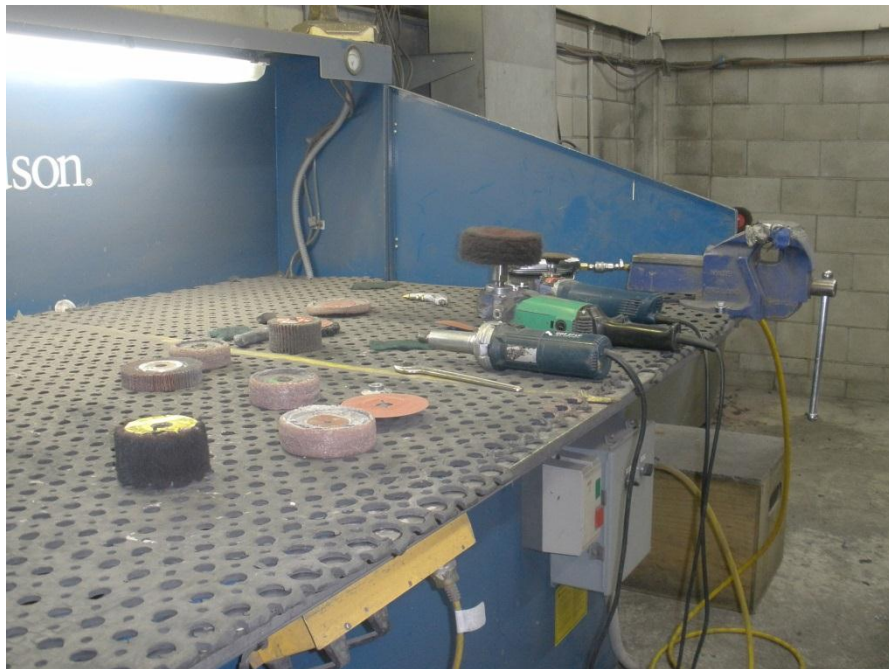
Plate 37: The extractor bench in the polishing room and various polishing wheels and pieces of equipment.
