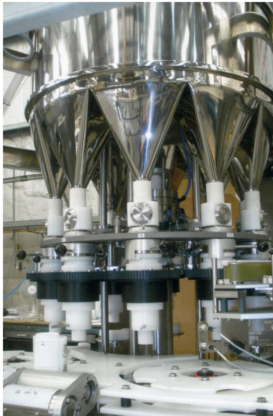
Plate 36: The tea filler - for filling packets of leaf tea. As can also be seen, this machine includes components of both plastic and stainless steel.
