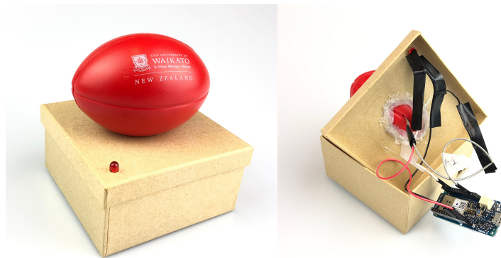
FIGURE 4.3: Preliminary study. Exterior: cardboard box with Rugby stress ball (left). Interior: Arduino MKR1000, FSR sensor, and LED (right), built according to the circuit diagram in Figure 4.2.
