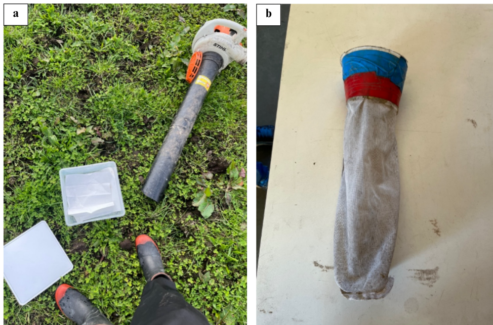
Figure A2.1 Field collection setup for obtaining parasitised Sitona weevils. (a) Blower-vacuum used for suction sampling in white clover pastures, alongside the collection container used to transfer debris to the laboratory; (b) Mesh collection pouch fitted that is fit to blower-vacuum nozzle for trapping weevils and pasture debris.
