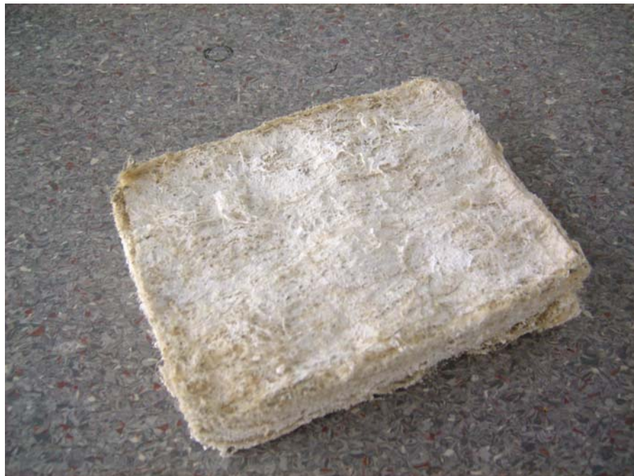
Figure 3.13 Solution mixed hemp fibre mat containing loosely bound polypropylene precipitates.
