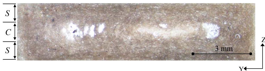
Figure 4.29 Macroscopic view of a test specimen cross-section showing a distinct core layer ( C ), and two skin layers ( S ).
