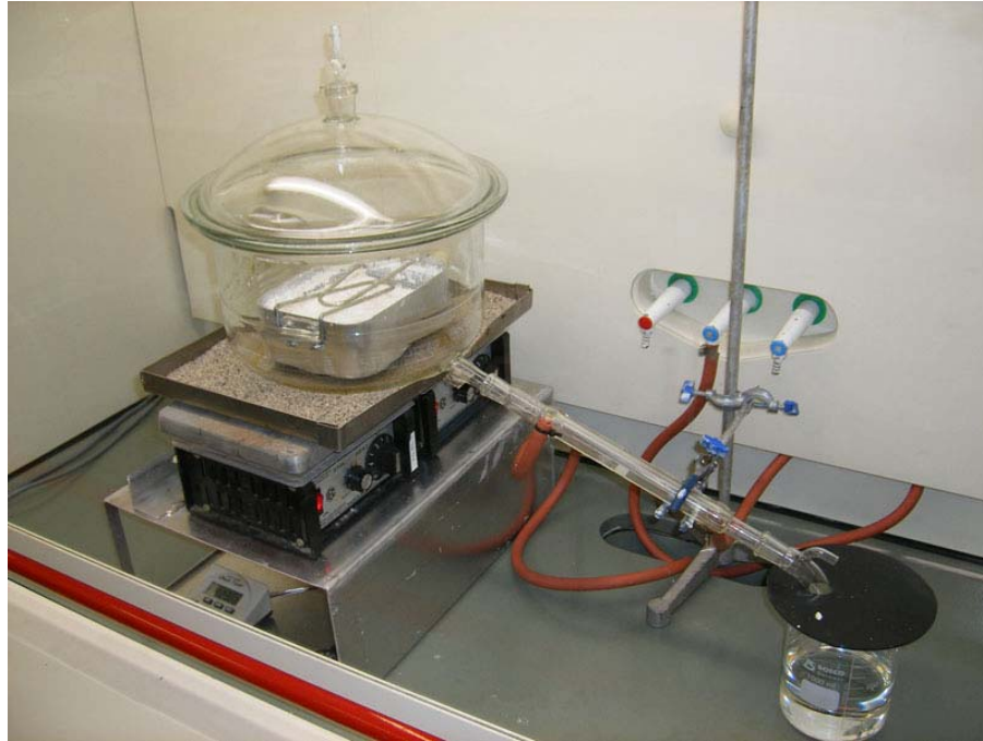
Figure 3.12 Solution mixing apparatus including evaporating tray, solvent evaporator and Liebig condenser.
