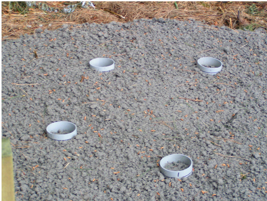
Figure 5.1. PVC collars inserted in Tasman primary solids (TPS) containing 126 g dw of TPS. Collars were raised (offset) 2.5cm above the surface of the solids.
