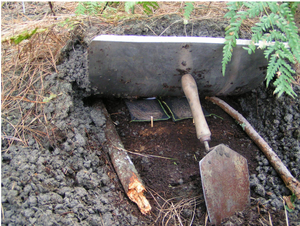
Figure 5.2. Needle litterbags were placed in the buried litter layer by inserting a metal sheet between waste solids and litter layer which was tilted up to allow access while causing minimal disturbance.
