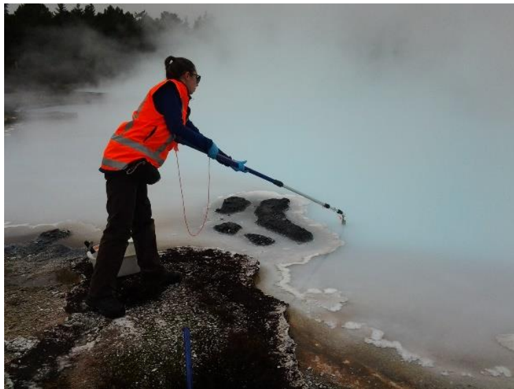
Figure 2.2: Sampling procedure using specialized water column sampler and personal protective equipment at Ohaaki geothermal field
