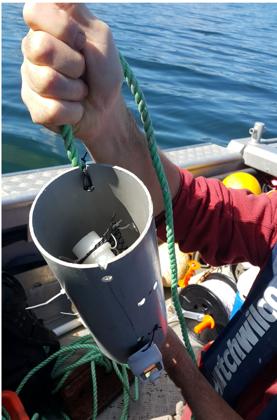
Figure 4. DGTs housed in a PVC pipe with temperature loggers to be suspended 5 meters above sediment and 5 meters below water surface
