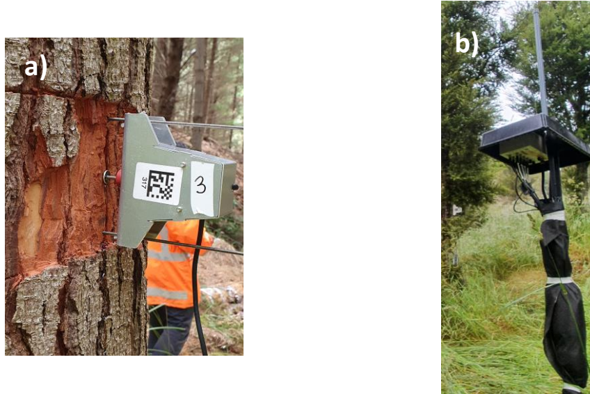
Figure 2.3: An electronic point dendrometer in one of the Pinus radiata plots (a), showing the steel button and scraped bark. A data logger (node) in one of the Lophozonia menziesii plots (b) to which the soil moisture sensors and dendrometers were connected.
