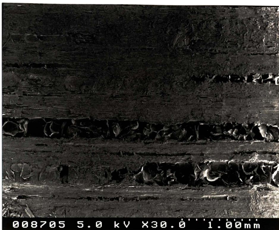
Figure 4.11 Side-grain wood from the interior surface of a barrel
