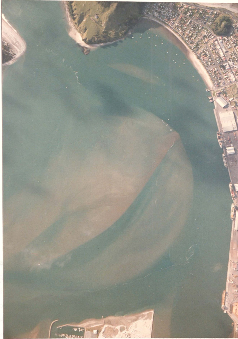
Plate 5.1 - Aerial photo of the Tauranga Harbour entrance taken in THS, August 1984. Waves ( L \approx 120\text{m} ) are propagating across Central Bank with some diffraction occurring in the vicinity of Pilot Bay.
