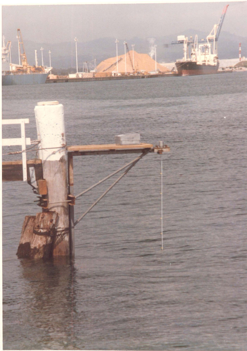
Plate A3.1 - The SUBTLE recording system as deployed on the southern BOPHB Tug Berth, Tauranga Harbour.
