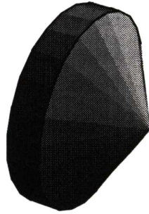
Figure 4-6. Schematic of the flat cone lens (axicon) used in the radial optics configuration.
