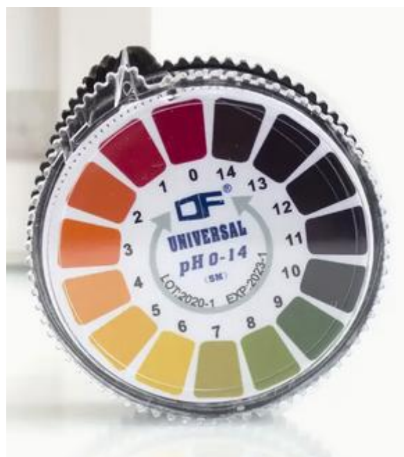
Figure 33 An example of a pH indicator product with a pH-sensitive dye.
