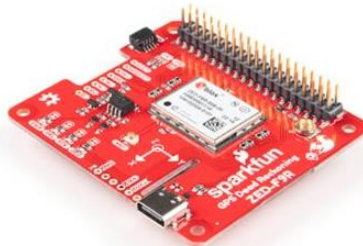
Figure 3.7: The u-blox ZED-F9R-00B module.
