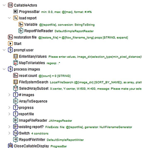
Figure 3.29: ADAMS structure with control actors and sub-actors for annotating objects.
