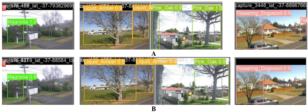
Figure 4.9: Comparative visualization of urban tree species detection during the validation phase by A. YOLOv5m and B. YOLOv8m.
