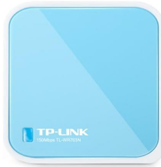
Figure 3.8: The TP-Link TL-WR703N Wi-Fi router.
