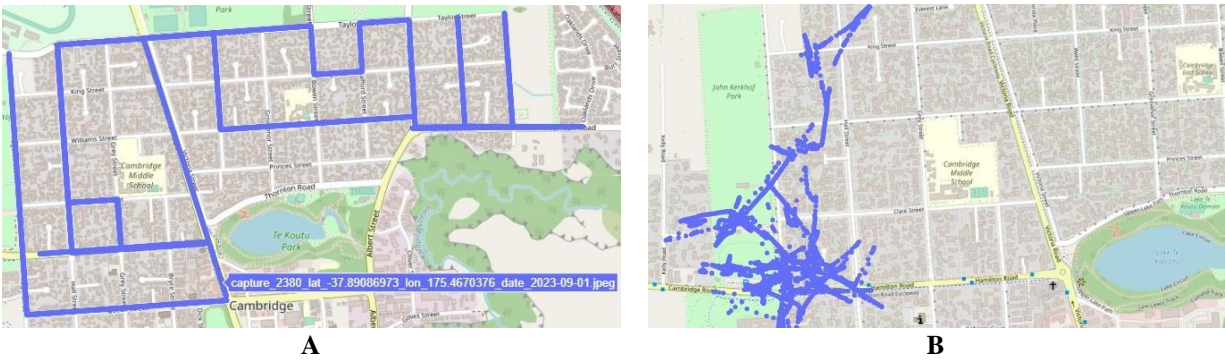
Figure 3.22: Comparative GPS coordinates from two datasets have been collected at different times from the same routes in Cambridge; A. Blue points represent GPS coordinates that are completely correct, and B. Blue points represent GPS coordinates that are completely wrong.
