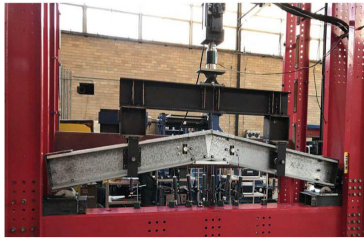
Figure 2-18 Photograph of the laboratory test set-up of apex joints Rinchen and Rasmussen (2019b)
