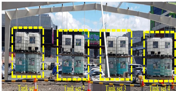
(a) Photograph of the portal frame test
