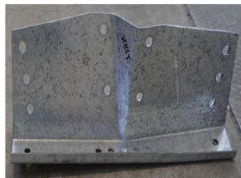
(b) Buckling failure of apex bracket
