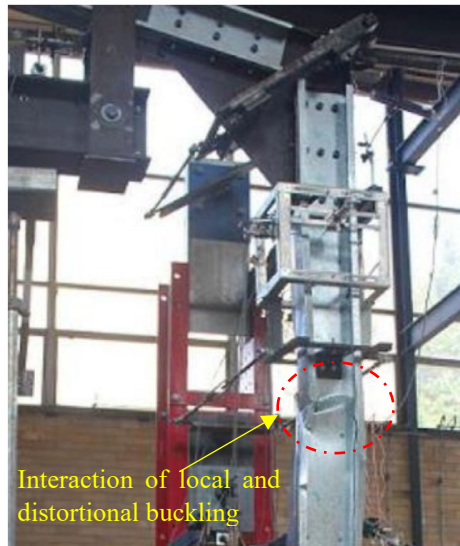
(b) Deformed shape of the column at failure
