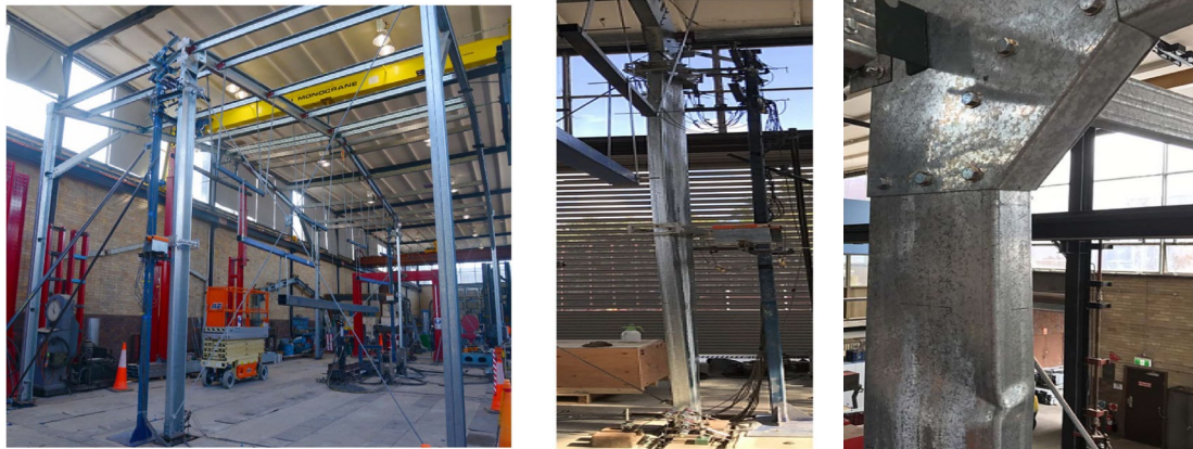
(a) Experimental test setup (b) Large displacements due to torsion (c) Local buckling in the column
