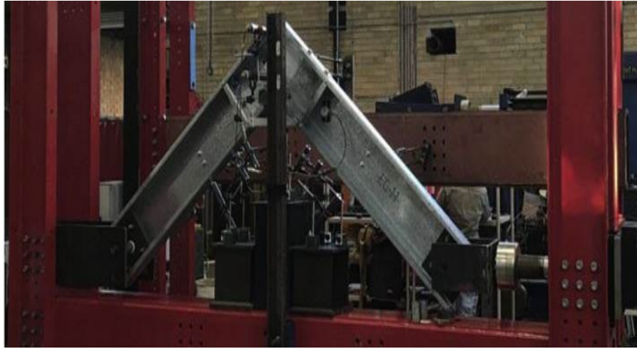
Figure 2-23 Photograph of the laboratory test set-up of eaves joint after Rinchen and Rasmussen (2019b)
