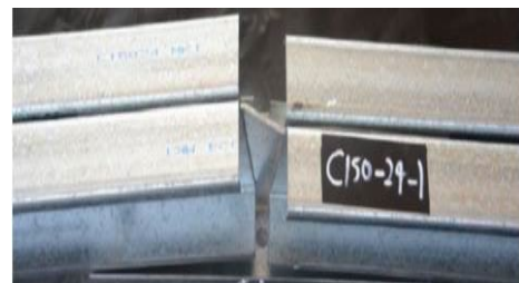
(b) Buckling of apex bracket
