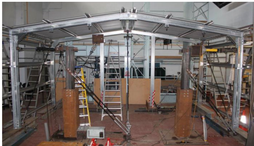
Figure 2-4 Experimental test setup CFS portal frame with back-to-back channels after Wrzesien et al. (2015)
