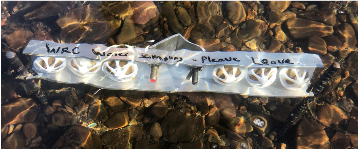
Figure 3-2. Passive manifold housing with six plastic pods with Dacron filter within each pod.
