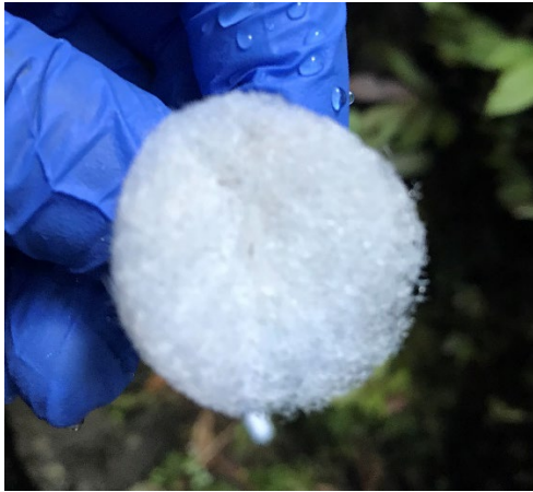
Figure 3-13. Clean passive filter after a 21 hour and 40-minute deployment at the upper tributary site (410_11), Manganui system.
