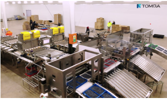
Fig. 5: KATO260 and LUCAi™, developed by BBC Technology, a popular blueberry sorting machine utilised by pack houses in New Zealand
