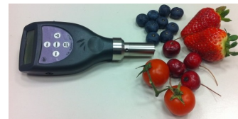
Fig. 4: Turoi 53215BE, a Non-destructive measurement of the firmness of soft fruit
