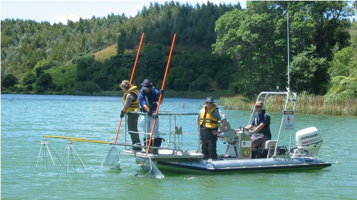
Figure 1. The electrofishing boat of the University of Waikato in Te Weta Bay, Lake Rotoiti, showing the fishing platform and anodes at the bow. Photo: Kim Young, DOC.
