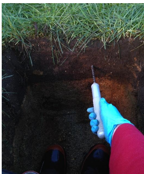
Figure 3.2: The penetration resistance of the soil being measured using a hand-held penetrometer.
