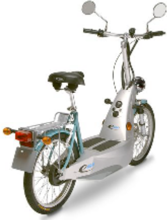
Fig. 2. 'eGO' 24V electric scooter.
