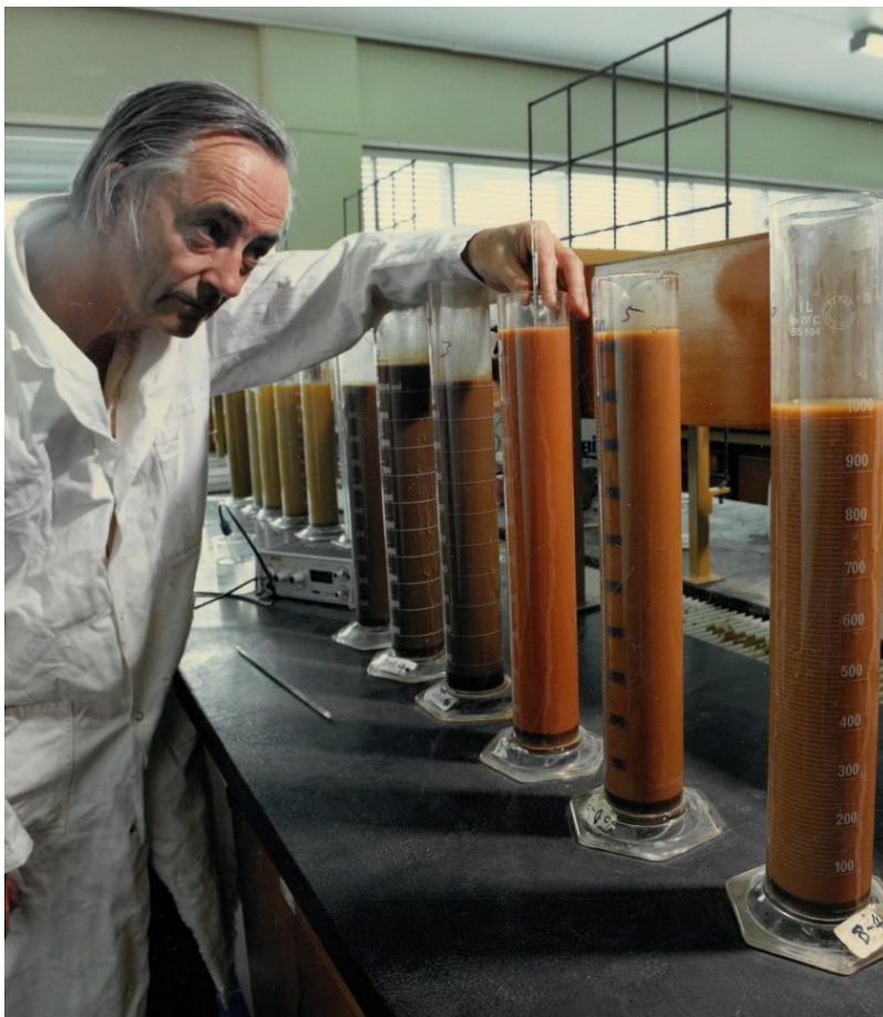
Bob in the lab measuring soil grain size distributions using the pipette method (1980s). Photo: (probably) Rex Julian or Ross Clayton.
