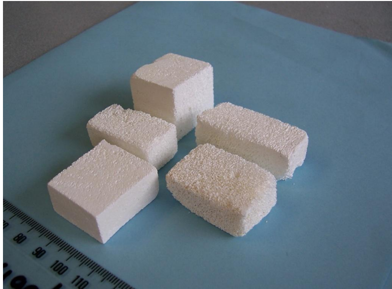
Figure 3-9 – SCBB sintered at 1000°C for 3 hours, cf. the original autoclaved samples in Figure 3-5.
