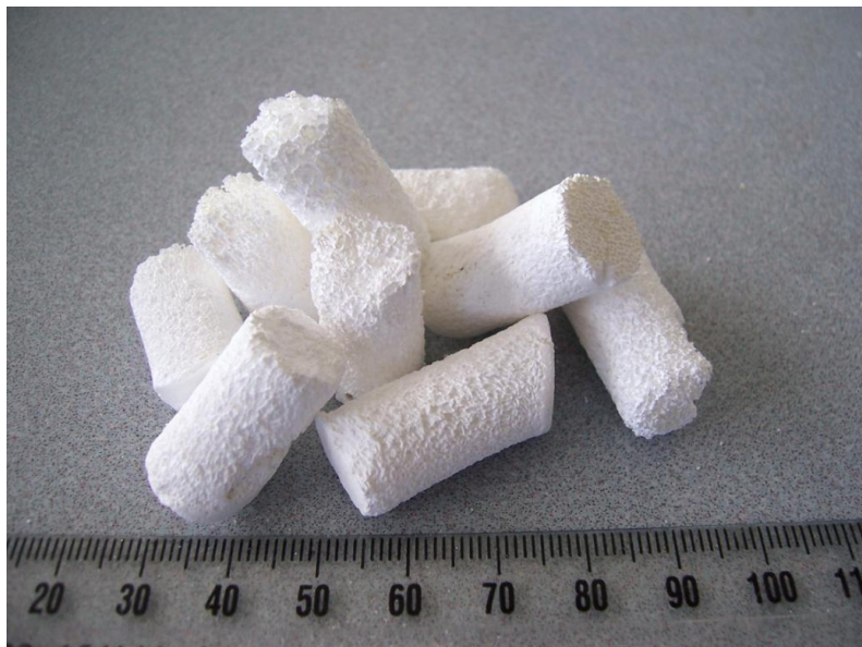
Figure 3-10 - Cylindrically shaped SCBB generated through autoclaving, coring and sintering processes.
