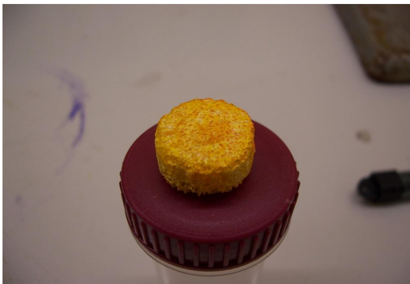
Figure 5-8 - Sintered cancellous bone having been infiltrated with chitosan and then the chitosan immobilised with 0.1 mol L -1 NaOH containing FITC.
