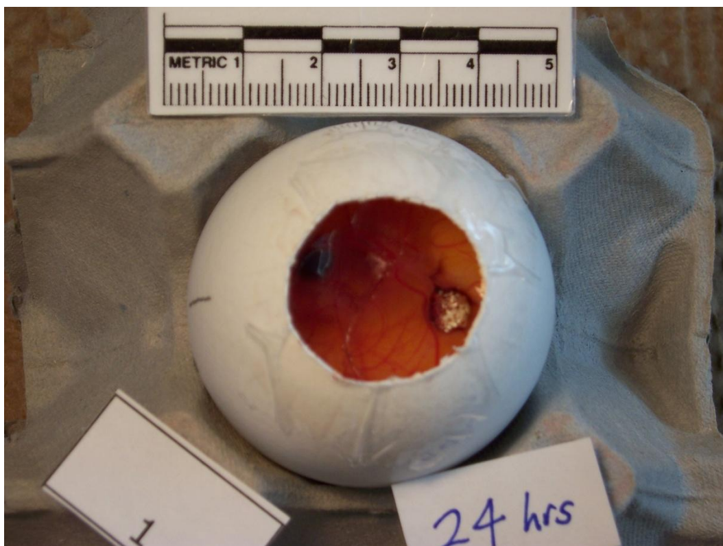
Figure 7-16– Photograph of BioSCBB-2 sample on CAM after 24 hours showing a ring of blood around the sample.
