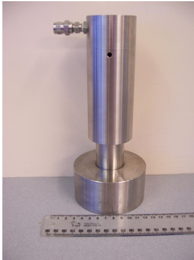
Figure 4-5 - Hydrostatic pressure vessel rated to 200 atm.
