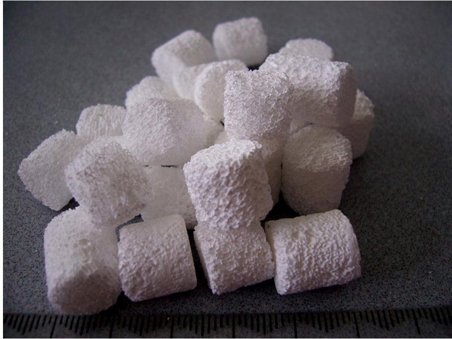
Figure 3-11 – Photograph of SCBB samples after having ends ground square.
