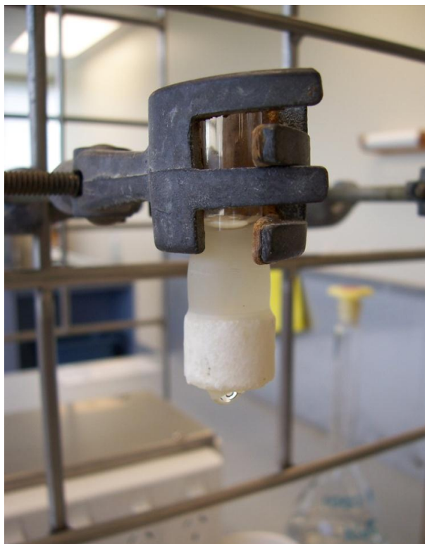
Figure 5-2 - Neutralisation of chitosan within SCBB by gravity induced flow of 0.1 \text{ mol L}^{-1} \text{ NaOH} solution through sample.
