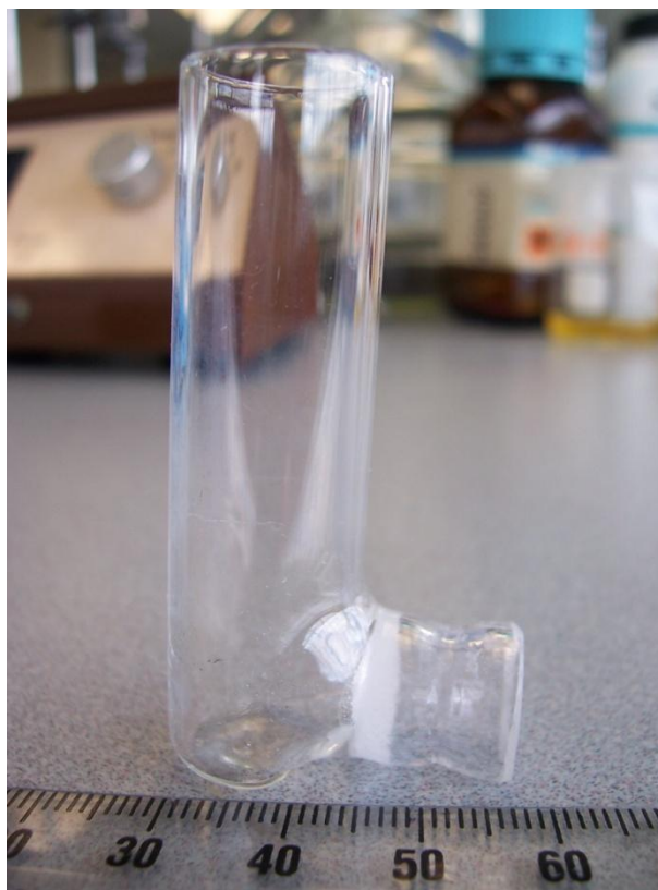
Figure 5-3 – Photograph of glass tubing making up a half-cell.
