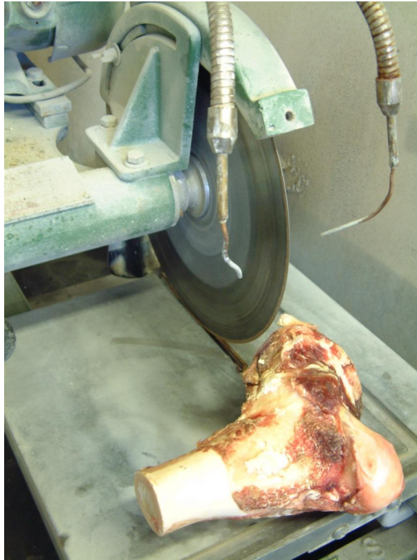
Figure 3-1 – Photograph of lapidary saw with bovine femoral bone.
