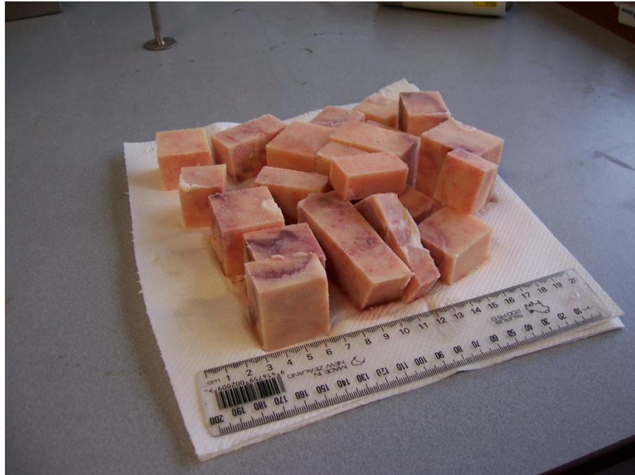
Figure 3-2 – Various shapes and sizes of raw cancellous bone prepared by lapidary saw.
