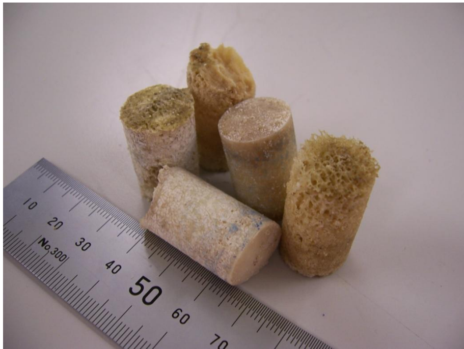
Figure 3-8 – Photograph of ‘dowels’ of autoclaved cancellous bovine bone generated by coring into sections of cancellous bone as shown above in Figure 3-7.
