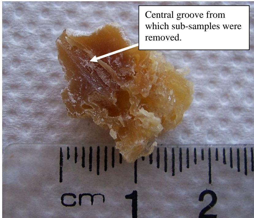
Figure 5-5 – Photograph of a solid lump of chitosan / CaP composite after being sectioned and sub-samples removed along a central groove.
