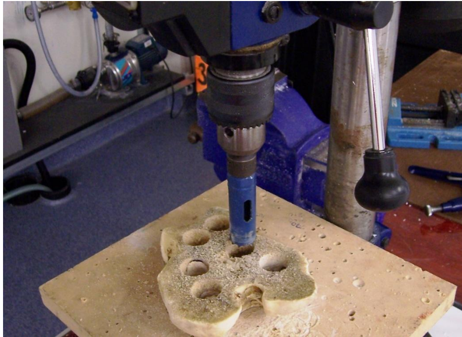
Figure 3-7 – Photograph of section of dried autoclaved bovine bone after being cored with Blu-Mol hole cutter.
