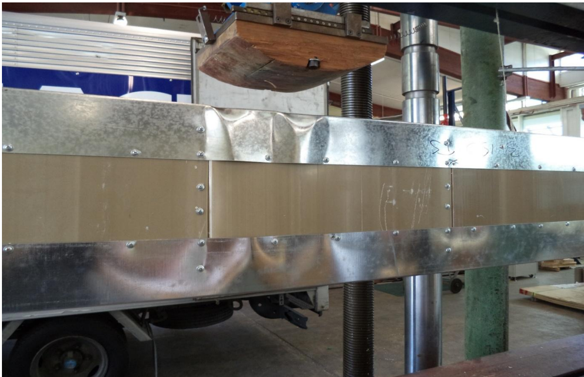
Figure 56-Local buckling of top steel channel during the three-point bending tests
