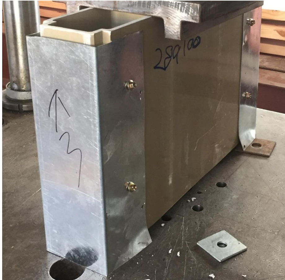
Figure 66-The steel U-section on the side buckling at the bottom
