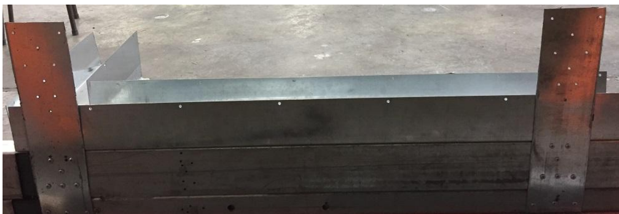
Figure 35-Overview of the 100mm \times 400mm \times 1.2 mm strap connected onto the steel joist
