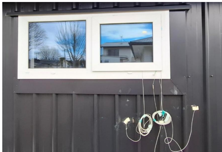
Figure 70-The Pico loggers set up on the outside of the wall
