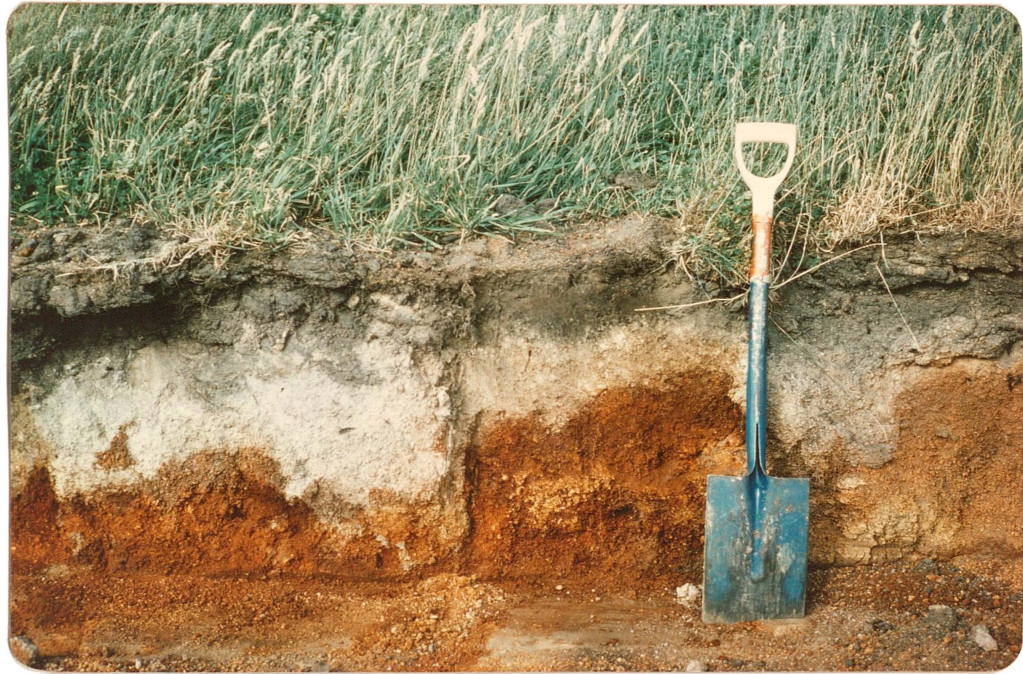
FIGURE 2.8 : Stratigraphic relationship between the dull yellowish brown and dark reddish brown lapilli of field class II at site 84, Whangamata South. (Spade is 1 metre in length).
