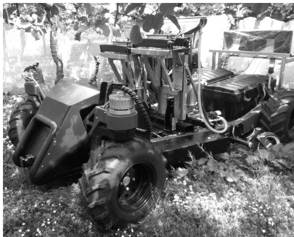
Figure 4 - Pollination system mounted on AMMP during experimental orchard trials
