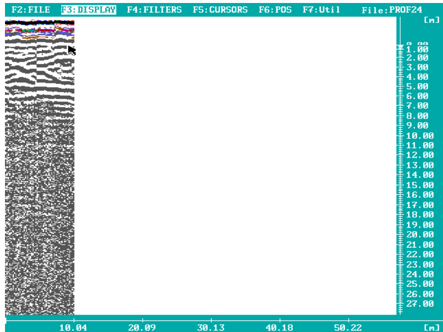
Radar gram of profile 24 trending NNW-SSW measured along the length of an observed limestone cave within the second bench of the High Grade unit, western side McDonald's Quarry (2007).
