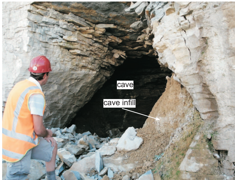
Figure 3.10 A limestone cave in the High Grade unit containing cave infill, typically a brown, moist, clay rich material. The infill is generally accumulated near the sides and at the bottom of the cave, western face.
