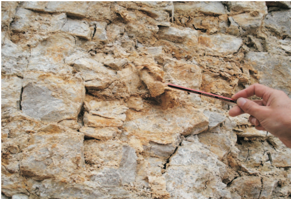
Figure 3.11 Palygorskite (creamy white clay mineral originally) on an exposed joint surface in the High Grade limestone unit. Palygorskite has leathery, flexible, and sheet like characteristics.
