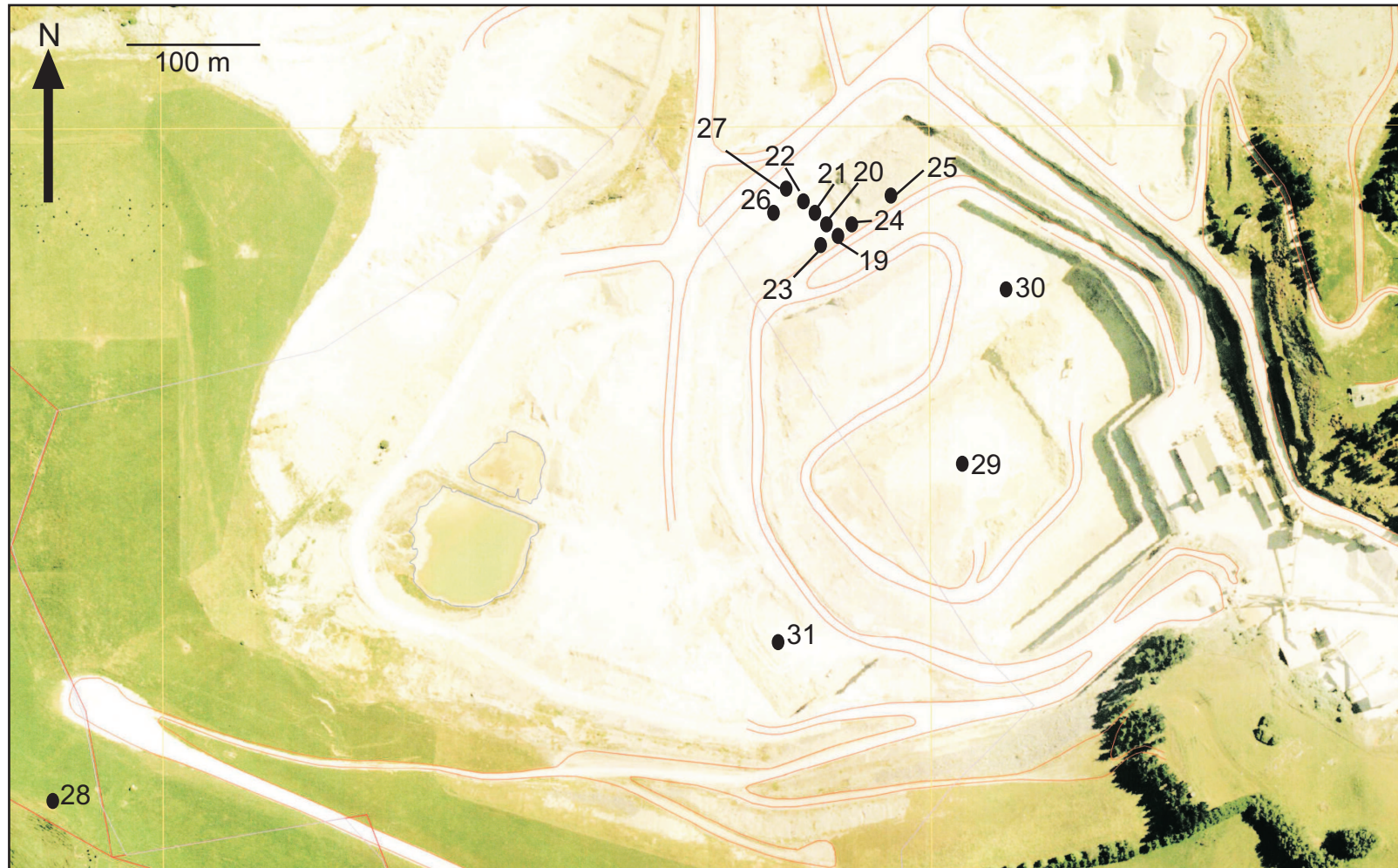
Figure 7.3 Transect location map for all profiles measured using ground penetrating radar in McDonald's Oparure Lime Quarry. The cluster of points (centre, top), are located on top of the upper High Grade bench below which a limestone cave is exposed. Aerial photo taken Feb 2007, sourced from McDonald's Lime Ltd..
