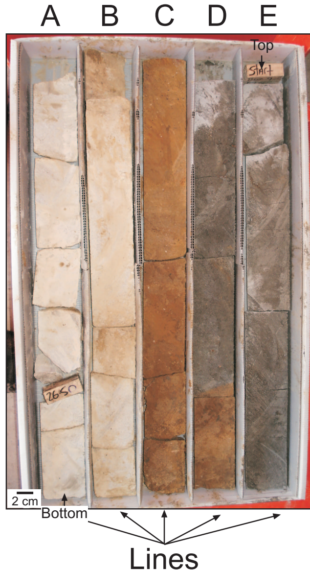
Figure 4.13 Box lines labelled by the letters A-E used in the discontinuity logging exercise for each box of cores, showing the top of the core (top right) and bottom of the core (bottom left).
