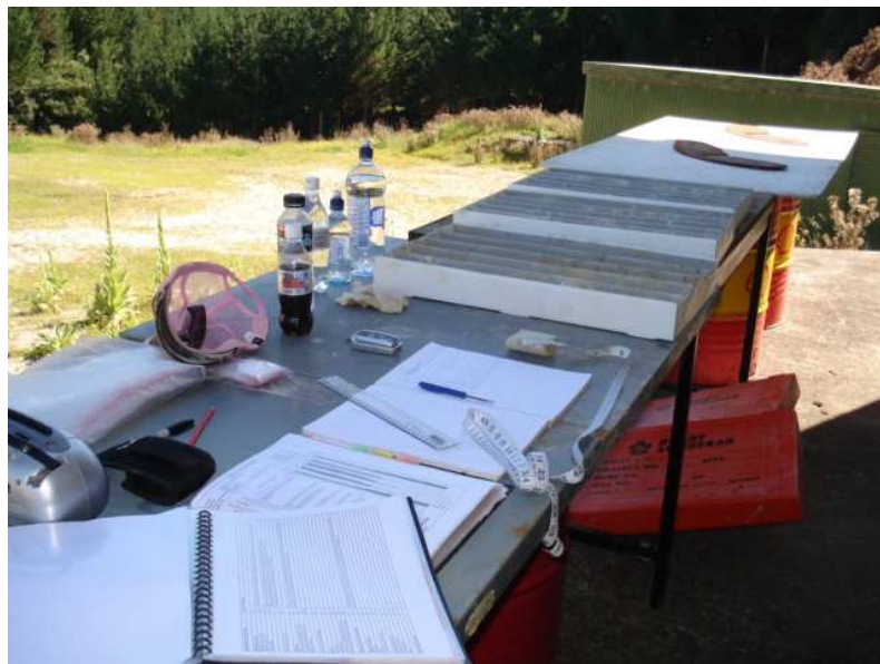
Figure 4.11 Tables set up outside the core shed for logging discontinuities in cores BH501, 502, and 503.
