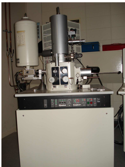
Figure 1 Hitachi Field Emission SEM instrument model S-1400 at the University of Waikato.
