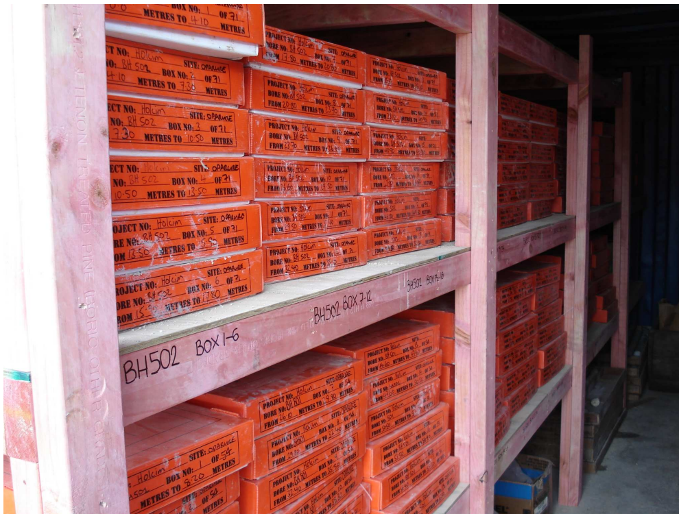
Figure 4.2 Photo from inside core shed showing boxes of core from drill hole BH502.
