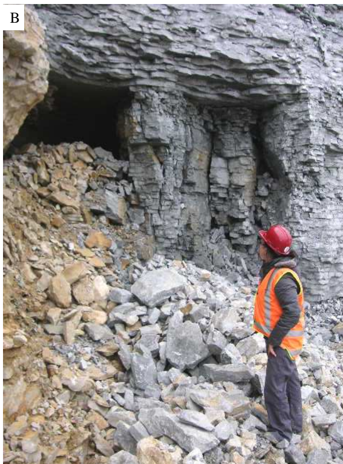
Figure 7.4 (A) Photo of the western side of the quarry (looking west) showing the location of the main limestone cave exposed within the second (upper) bench of the High Grade unit. (B) Photo showing entrance to limestone cave within the second bench of the High Grade unit. Previous blasting (indicated by rubble surrounding entrance) has exposed the cave.
