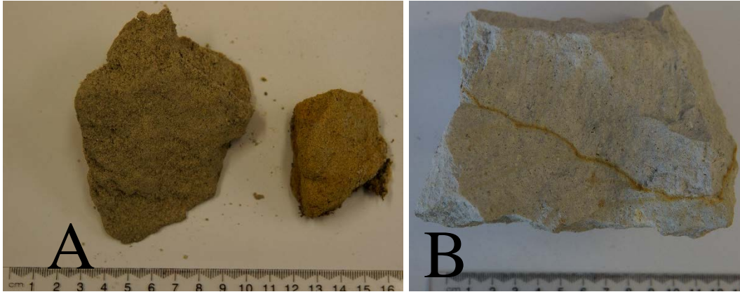
Figure 4.17: A: Facies W1 – the soft basal facies of the Waikino Ignimbrite (from the Waikino Quarry, Locality 4). B: Facies W2 – the moderately welded facies of the Owharoa Ignimbrite.
