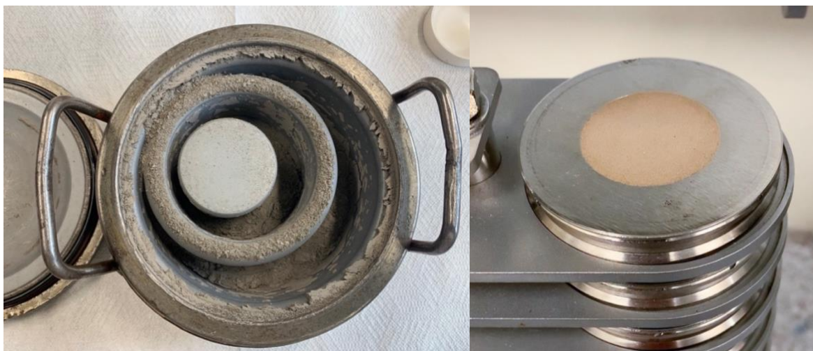
Figure 20: Preparation of soil samples for clay mineralogy analysis by X-ray diffraction. Left: Sample crushed within the tungsten-carbide ring mill. Right: Crushed soil prepared into a pressed palate mould.
