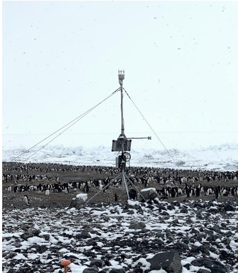
Figure 13: Automated weather station set up within the Cape Bird northern colony from the 28 th of December 2023 to the 10 th of January 2023.
