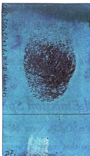
Figure 4.7 A fingerprint developed by a drag in 1.6 \times 10^{-3} M \text{CuPc}(\text{SO}_2\text{Cl})_4 ethanol solution, followed by ninhydrin; note approximately 1 year since print developed
