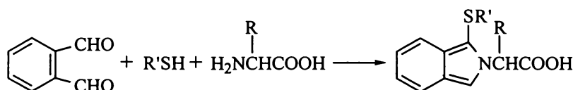
Scheme 1.7 Reaction of o -phthalaldehyde with amino acids [12]
